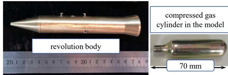
Figure 3. Test model and high-pressure cylinder.
