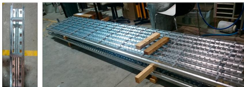
**Figure 1.** The reinforcement system and the constituent elements: (a) graphical section detail and (b) upright column in tests.
