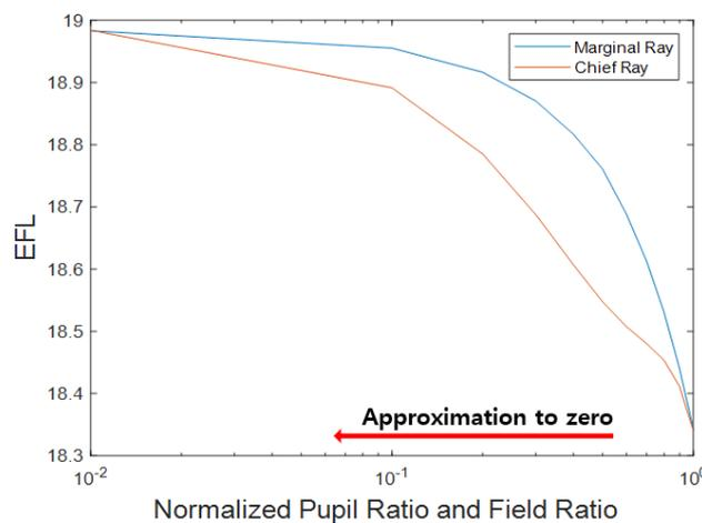
**Figure 7.** EFL change according to normalized pupil height for axial ray and normalized field ratio for chief ray.
