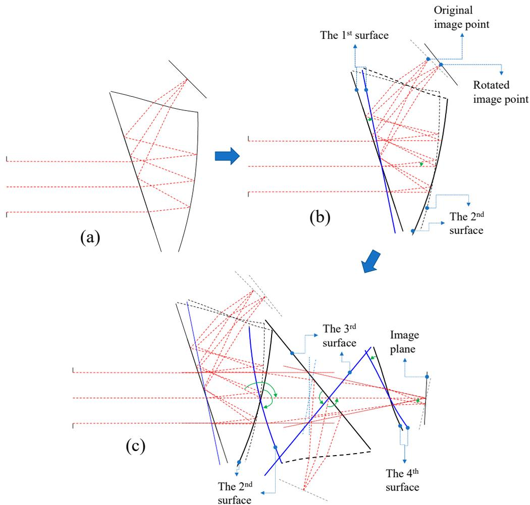
**Figure 4.** The rotated transformed optical layout such that the axial rays of the off-axis optical system are straight. (a) depicts the original optical system. (b) demonstrates that the entire optical system is rotated so that the axial ray on the optical axis refracted from the first surface becomes a straight line. (c) indicates the result of similarly rotating the axial ray on the optical axis to a straight line from the second surface to the last surface.
