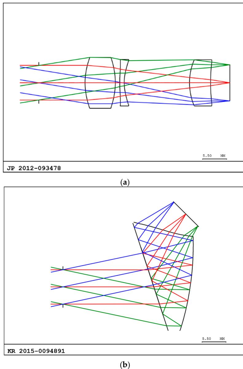
**Figure 1.** Eyepiece optics with the same specifications. (a) Examples of rotationally symmetric (on-axis) optical systems, (b) examples of asymmetric (off-axis) optical systems.
