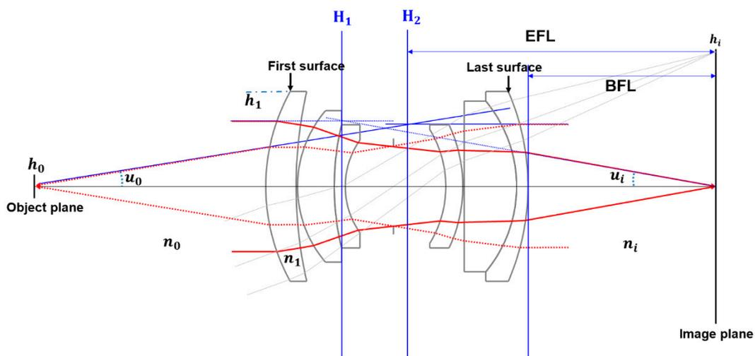
Figure 3. The optical layout for an on-axis optical system.
