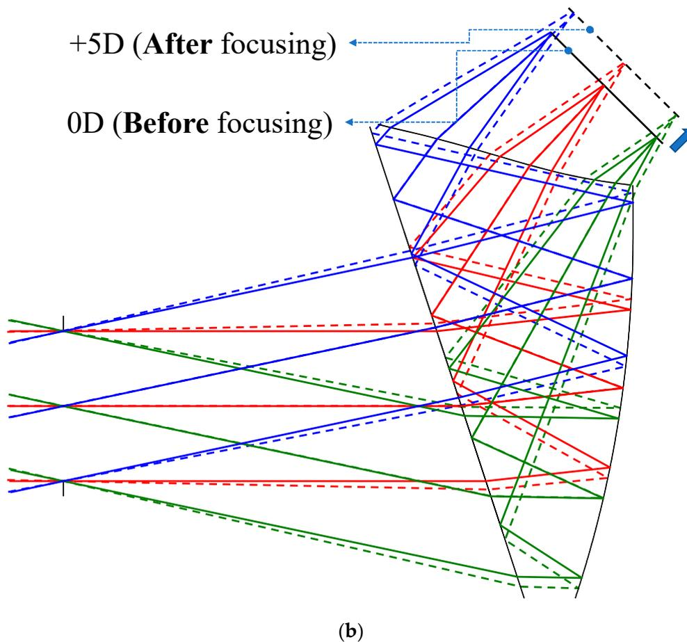
**Figure 6.** Adjusting the focus of the eyepiece. (a) The optical paths when changing from 0 to  $-5$  D and (b) 0 to 5 D.
