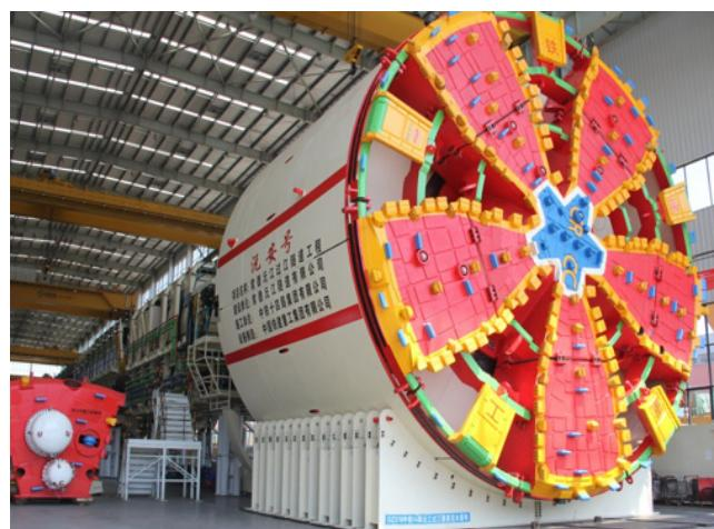
**Figure 9.** Yuanan shield machine cutter of Yuanjiang Tunnel.
