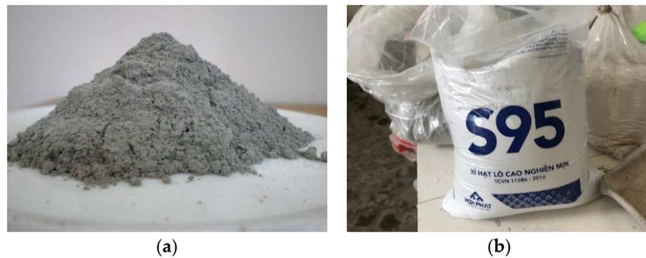
**Figure 2.** Fly ash and granulated blast furnace slag: (a) fly ash; (b) granulated blast furnace slag.
