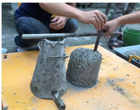
**Figure 6.** Slump test of GPC.
