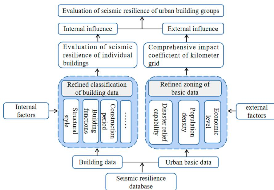
**Figure 4.** Flow chart for seismic resilience evaluation of urban building groups through classification and zoning.
