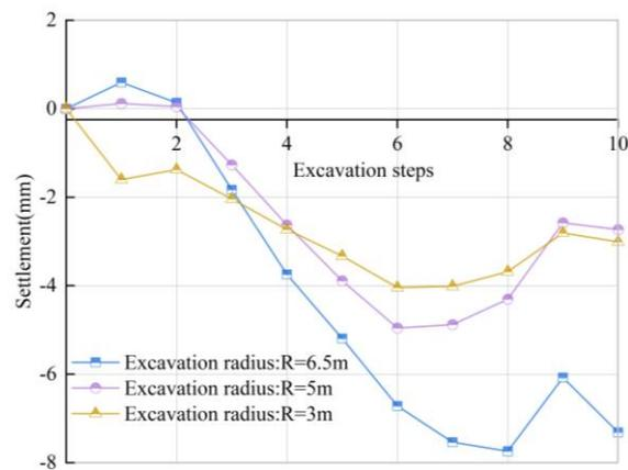
**Figure 16.** Influence of excavation radius on the longitudinal deformation of the ground surface.
