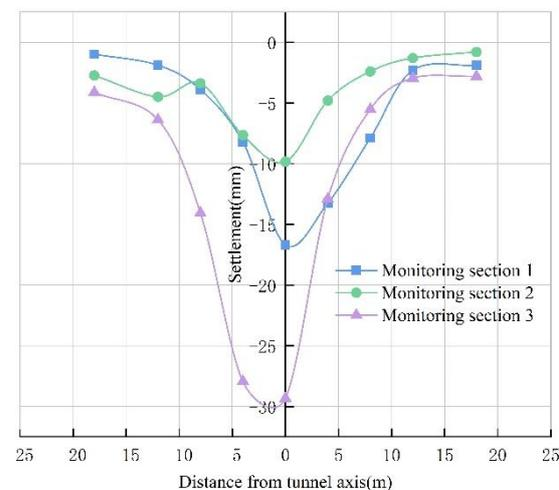
**Figure 4.** Lateral surface settlement trough caused by tunnel excavation.
