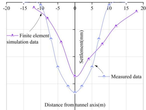
**Figure 7.** Comparison of monitoring data and numerical model surface transverse curve.
