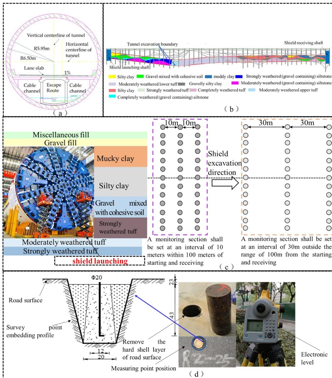
**Figure 1.** Overview of the shield test section; (a) Tunnel design effect diagram; (b) Tunnel excavation geology and roadside diagram; (c) Measuring point layout diagram; (d) Measuring point burying and monitoring construction diagram.
