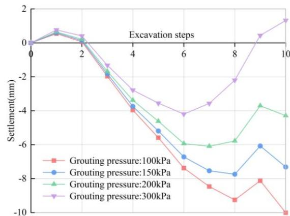
**Figure 14.** Influence of grouting pressure on the longitudinal deformation of the ground surface.
