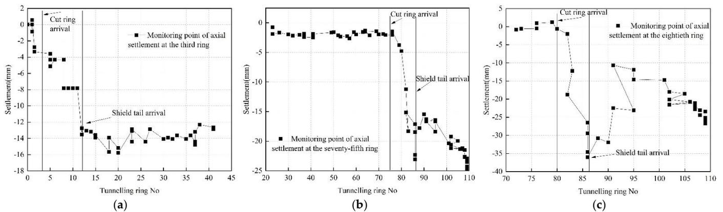
**Figure 2.** Surface settlement monitoring curve (a) Surface settlement duration curve of the axis at ring 3; (b) Surface settlement duration curve of the axis at ring 75; (c) Surface settlement duration curve of the axis at ring 80.
