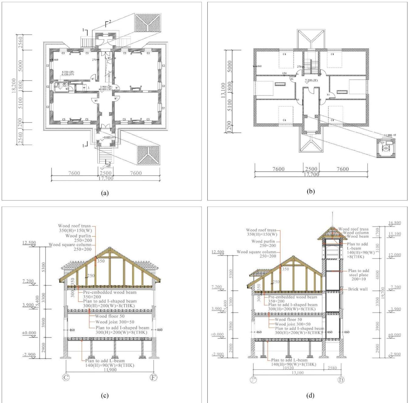
**Figure 10.** Structural elements of the bell tower (source: author). (a) The first and second floor plan (b) The third floor plan. (c) Building structure element (1–1 section diagram) (d) Building structure element (2–2 section diagram).
