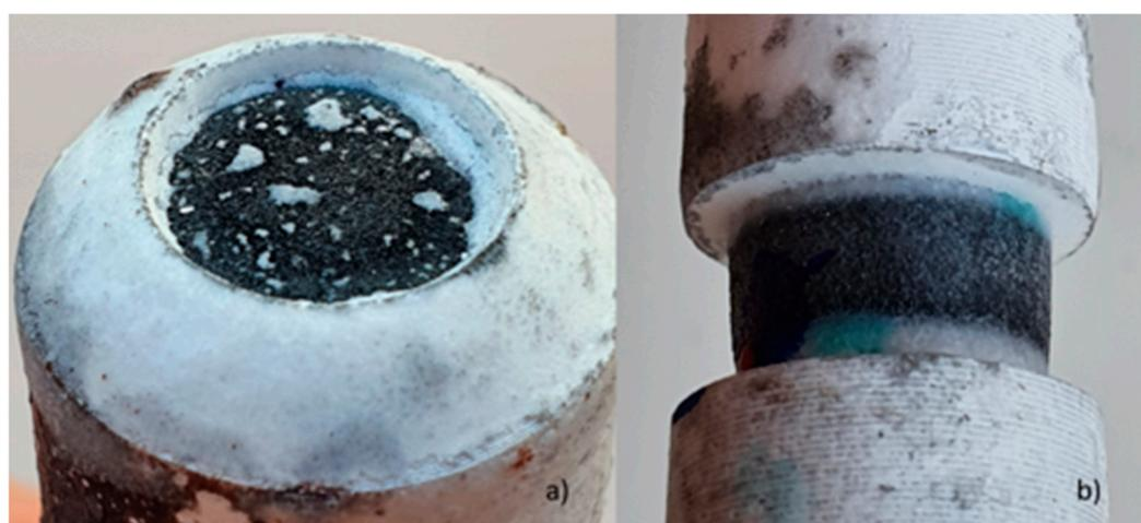
**Figure 13.** Images of anodes after experiment: (a) horizontal anode and (b) vertical anode.
