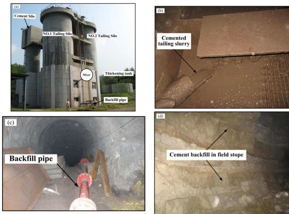
**Figure 1.** The cemented tailings backfill system in the Daye Iron Mine: (a) cemented tailings backfill plant; (b) cement tailings slurry; (c) transportation pipe for backfill slurry; (d) backfill in field stope.
