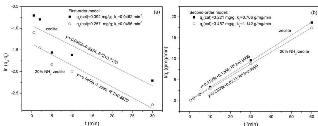
**Figure 13.** Plots of pseudo-first-order (a) and pseudo-second-order kinetic models (b) for adsorption of naphthalene onto zeolite and the 20% amino functionalized zeolite sample.
