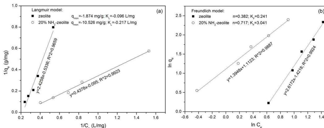
Figure 15. Langmuir (a) and Freundlich (b) plots for adsorption of naphthalene onto the zeolite and amino functionalized zeolite samples.
