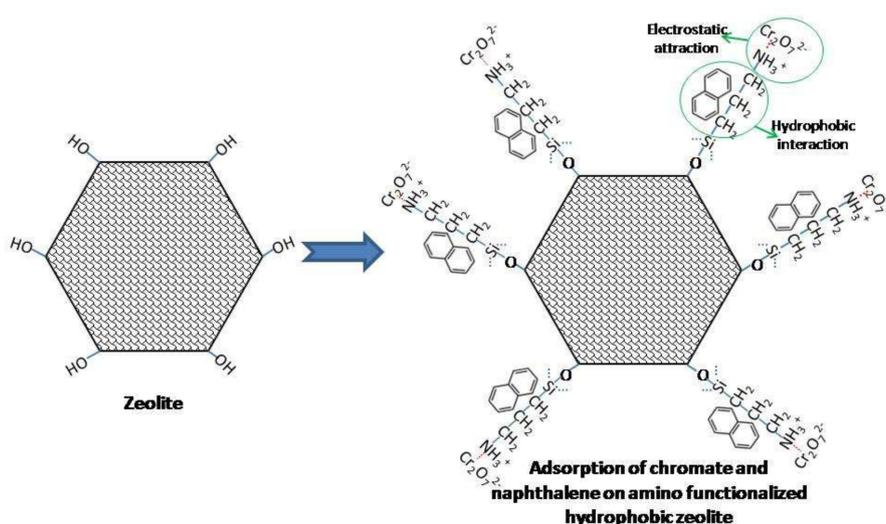
**Figure 16.** Schematic for modification of natural zeolite and the adsorption process of the amino functionalized hydrophobic zeolite on chromate and naphthalene.
