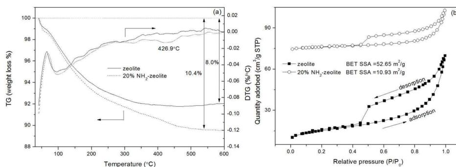
**Figure 4.** Thermal gravimetric and differential thermal gravimetric analysis (TG-DTG) curves (a) and  $N_2$  adsorption-desorption isotherms (b) of zeolite and 20% amino functionalized zeolite sample; the isotherms for 20% amino functionalized zeolite are vertically offset by around  $75 \text{ cm}^3/\text{g}$ .
