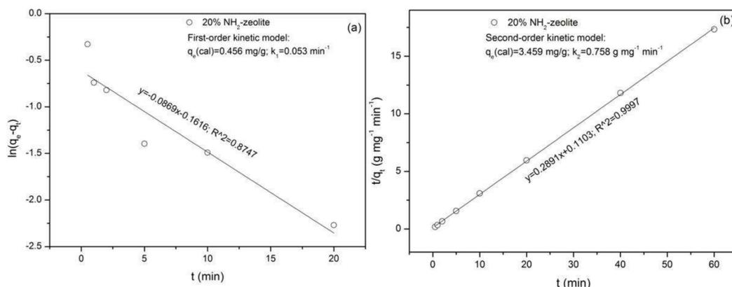
**Figure 8.** Plots of pseudo-first-order (a) and pseudo-second-order kinetic (b) models for adsorption of chromate ions onto 20% amino functionalized zeolite sample.
