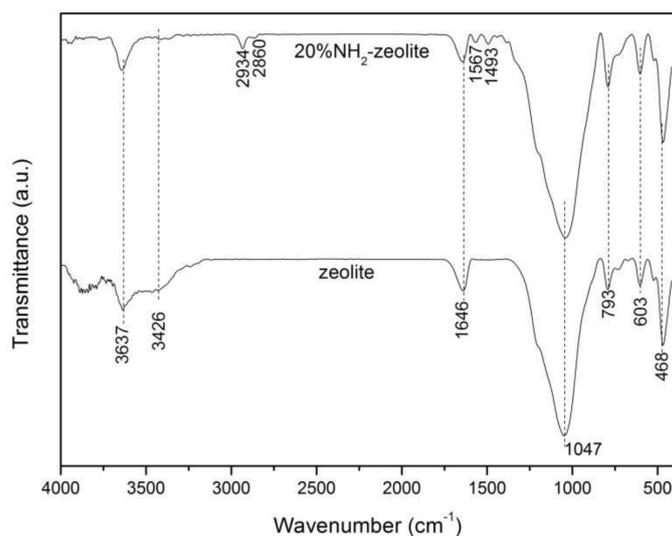
**Figure 3.** Fourier transform infrared analysis spectra of zeolite and 20% amino functionalized zeolite sample.
