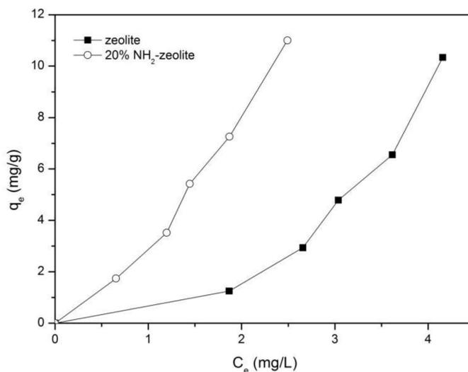
Figure 14. Isotherm for adsorption of naphthalene onto the zeolite and amino functionalized zeolite samples.
