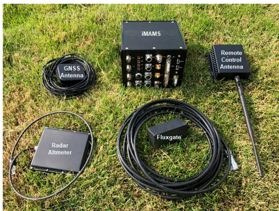
**Figure 1.** A typical set of components of iMAMS.
