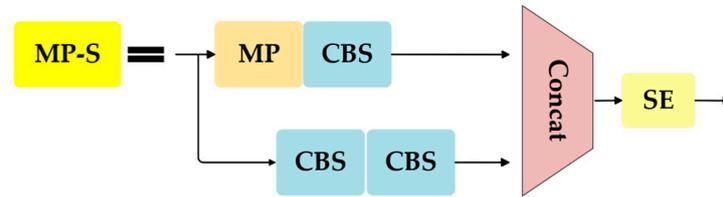
Figure 4. Structure of the MP-S module.
