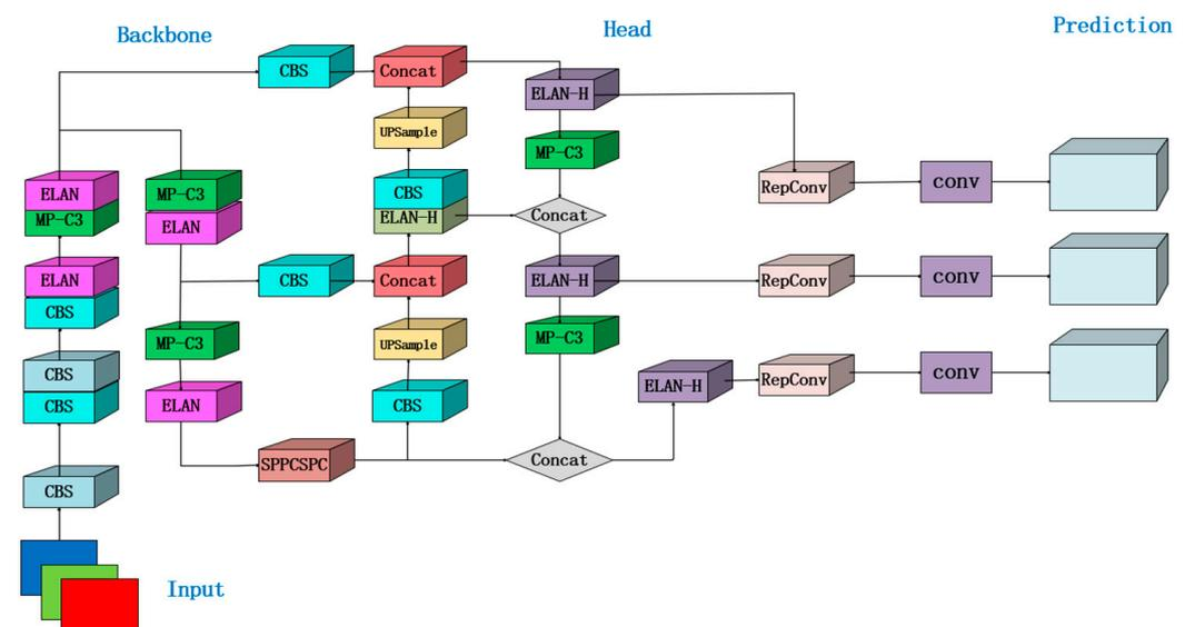
Figure 1. The network structure of YOLOv7.
