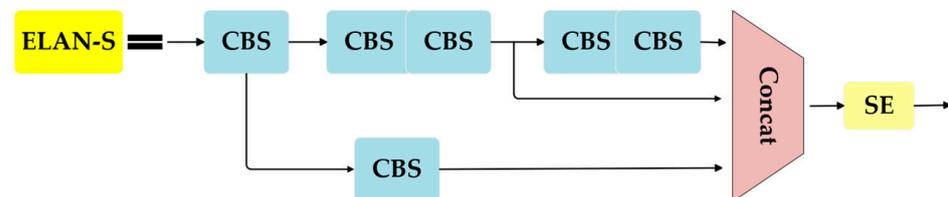
**Figure 3.** Structure of the ELAN-S module.
