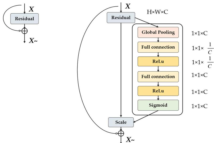
Figure 5. The structure diagram of the SE model.
