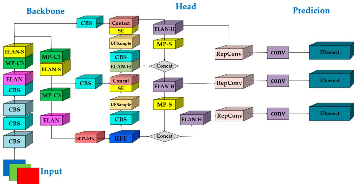
**Figure 2.** Structure of the proposed YOLO-SN network.
