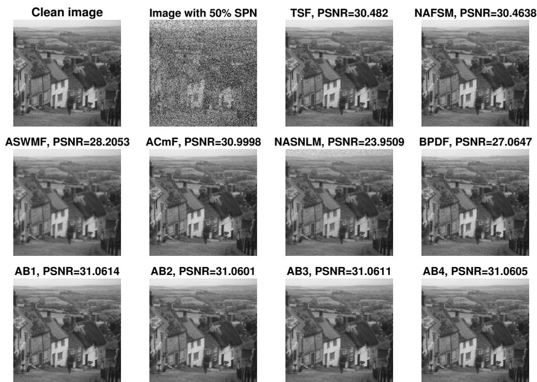
Figure 14. Comparison of the performance of different methods for salt-and-pepper noise ratio of 50%.
