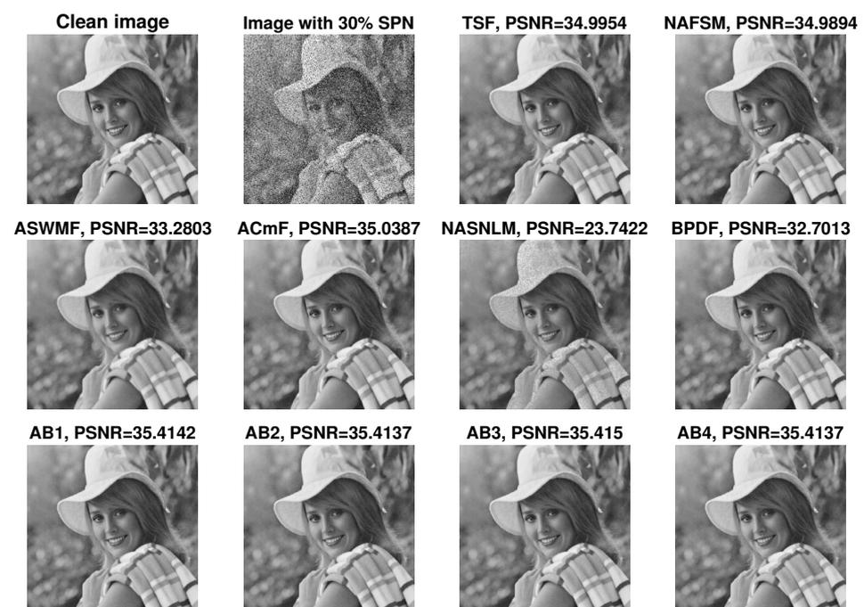
**Figure 3.** Comparison of the performance of different methods for salt-and-pepper noise ratio of 30% for Elaine.
