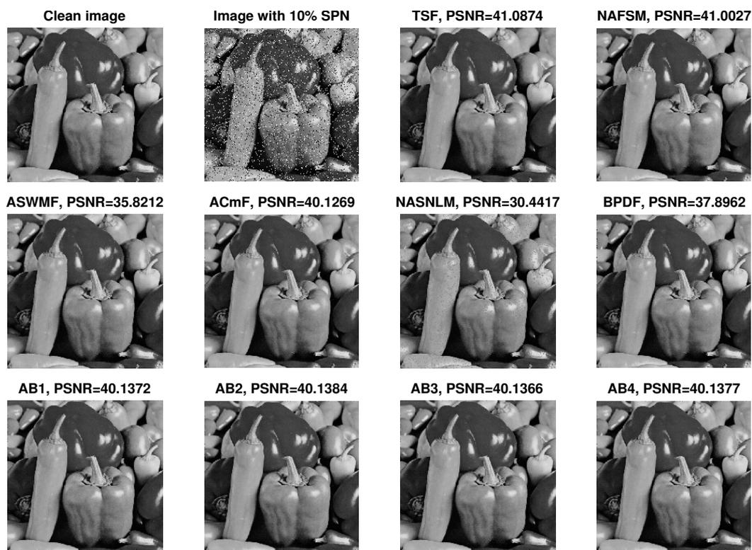
**Figure 7.** Comparison of the performance of different methods for salt-and-pepper noise ratio of 10% for peppers.
