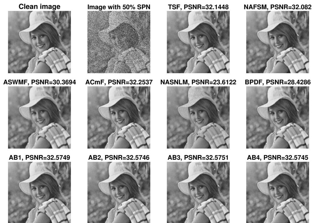
**Figure 4.** Comparison of the performance of different methods for salt-and-pepper noise ratio of 50% for Elaine.
