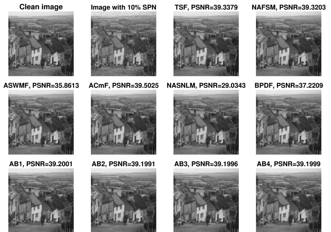
Figure 12. Comparison of the performance of different methods for salt-and-pepper noise ratio of 10%.
