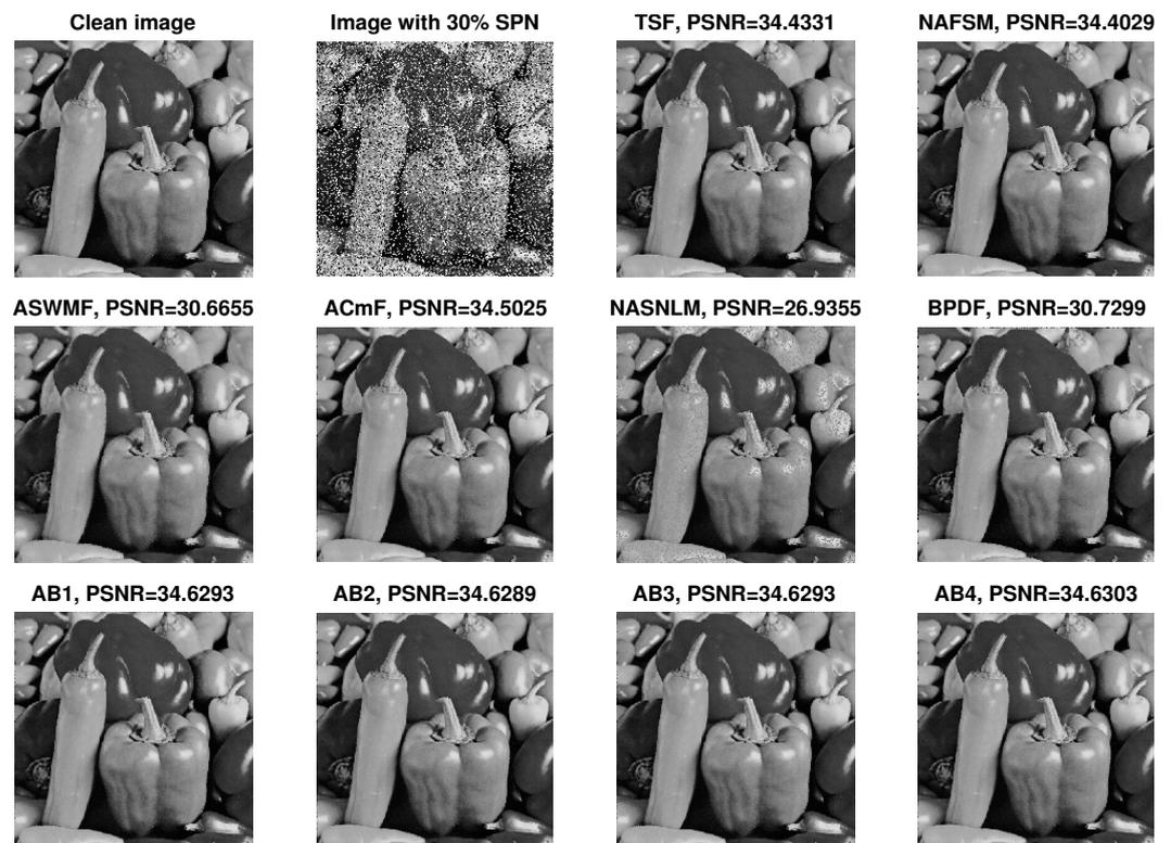
**Figure 8.** Comparison of the performance of different methods for salt-and-pepper noise ratio of 30% for peppers.
