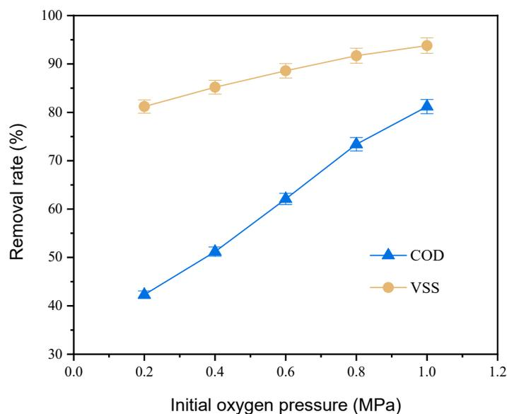
**Figure 6.** Influence of initial oxygen pressure on sludge degradation.
