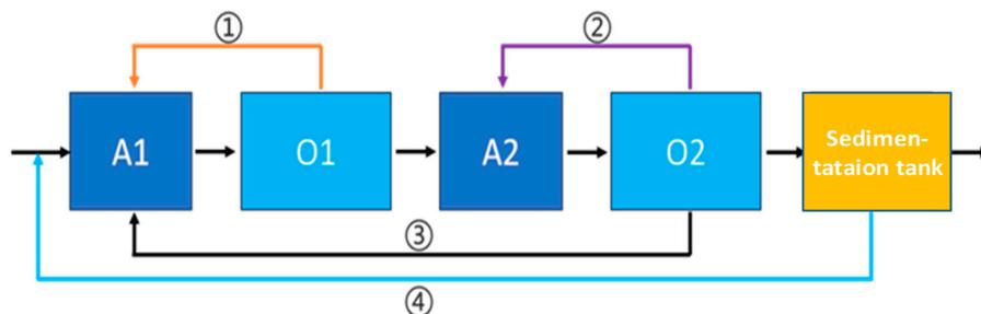
**Figure 1.** The process flow diagram of the simulated two-stage A/O process (① nitrification liquid reflux from primary aerobic tank to primary anaerobic tank; ② nitrification liquid reflux from secondary aerobic tank to secondary anoxic tank; ③ nitrification liquid reflux from secondary aerobic tank to primary anaerobic tank; ④ sludge reflux from sedimentation tank to primary anoxic tank).
