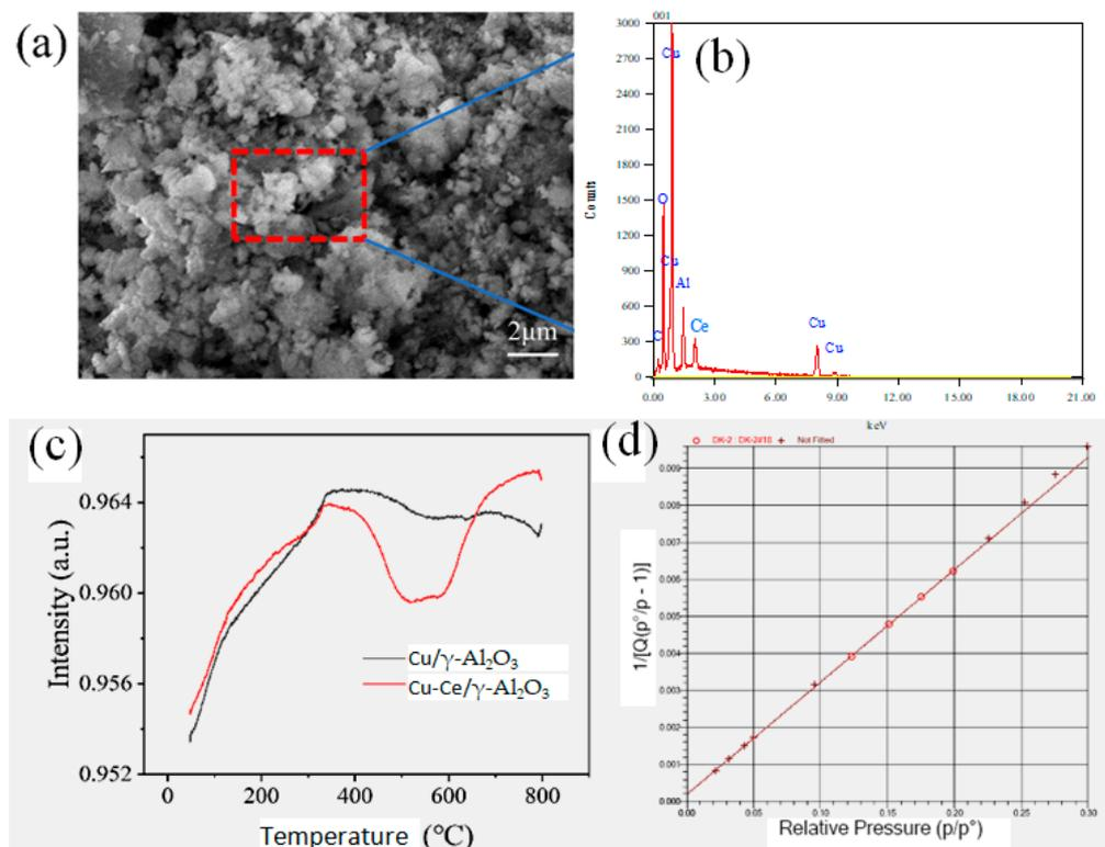
**Figure 2.** (a) SEM image of Cu-Ce/ $\gamma$ -Al<sub>2</sub>O<sub>3</sub> and (b) the corresponding content of elements; (c) temperature-programed oxidation spectra; (d) BET linear curve of Cu-Ce/ $\gamma$ -Al<sub>2</sub>O<sub>3</sub>.
