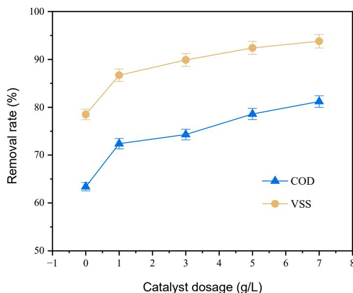
**Figure 3.** Influence of catalyst dosage on the sludge degradation.
