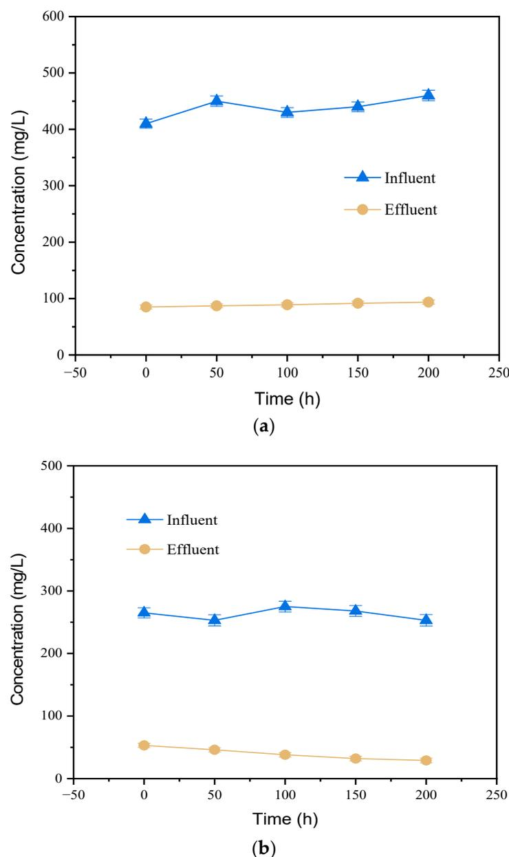
Figure 7. COD (a) and TN (b) concentrations in the influent and effluent.
