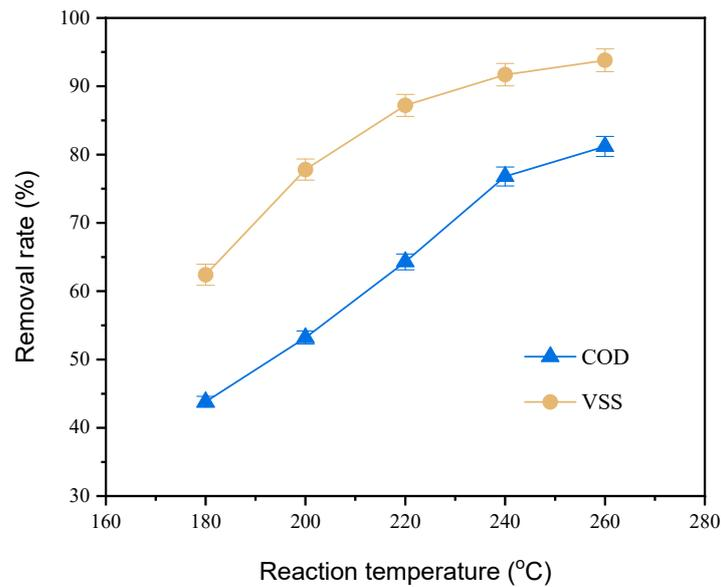
**Figure 4.** Influence of reaction temperature on sludge degradation.
