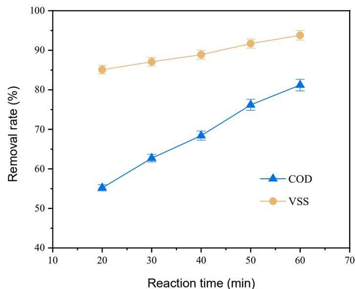
**Figure 5.** Influence of reaction time on sludge degradation.
