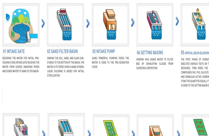
Figure. Busan Metropolitan city drinking water purification process ( busan.go.kr )
