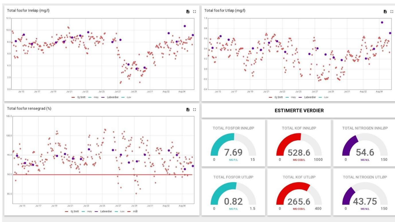
**Figure 6.** GUI dashboard presenting estimated values of TP influent and effluent along with lab-measured values for a period.
