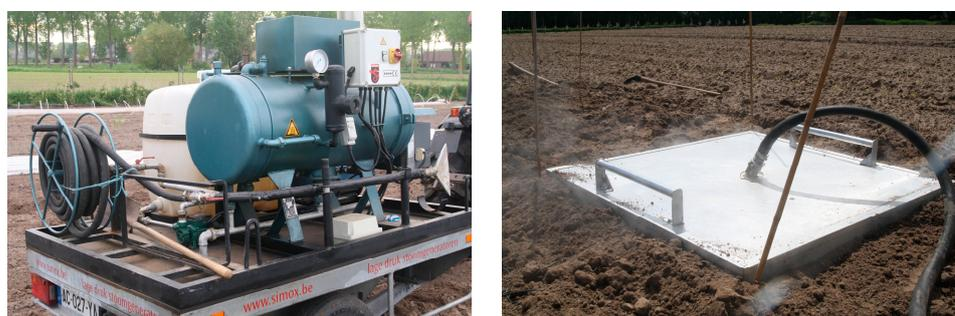
**Figure 2.** (Left): The steam generator, water tank, and flexible hose connected between the steam generator and the hooded application unit. (Right): The aluminum hooded application unit.
