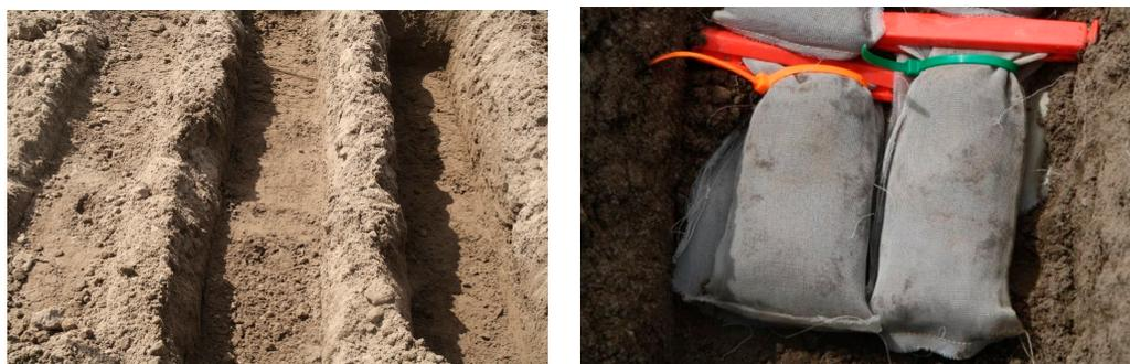
**Figure 3.** (Left): The gullies with depths of 5 cm (left), 15 cm (middle), and 25 cm (right). (Right): detail of the nylon bags which were laid in the gullies.
