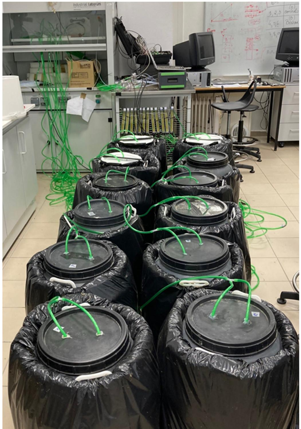
**Figure 1.** View of the pilot scale composting experiment and equipment used to measure gaseous emissions.
