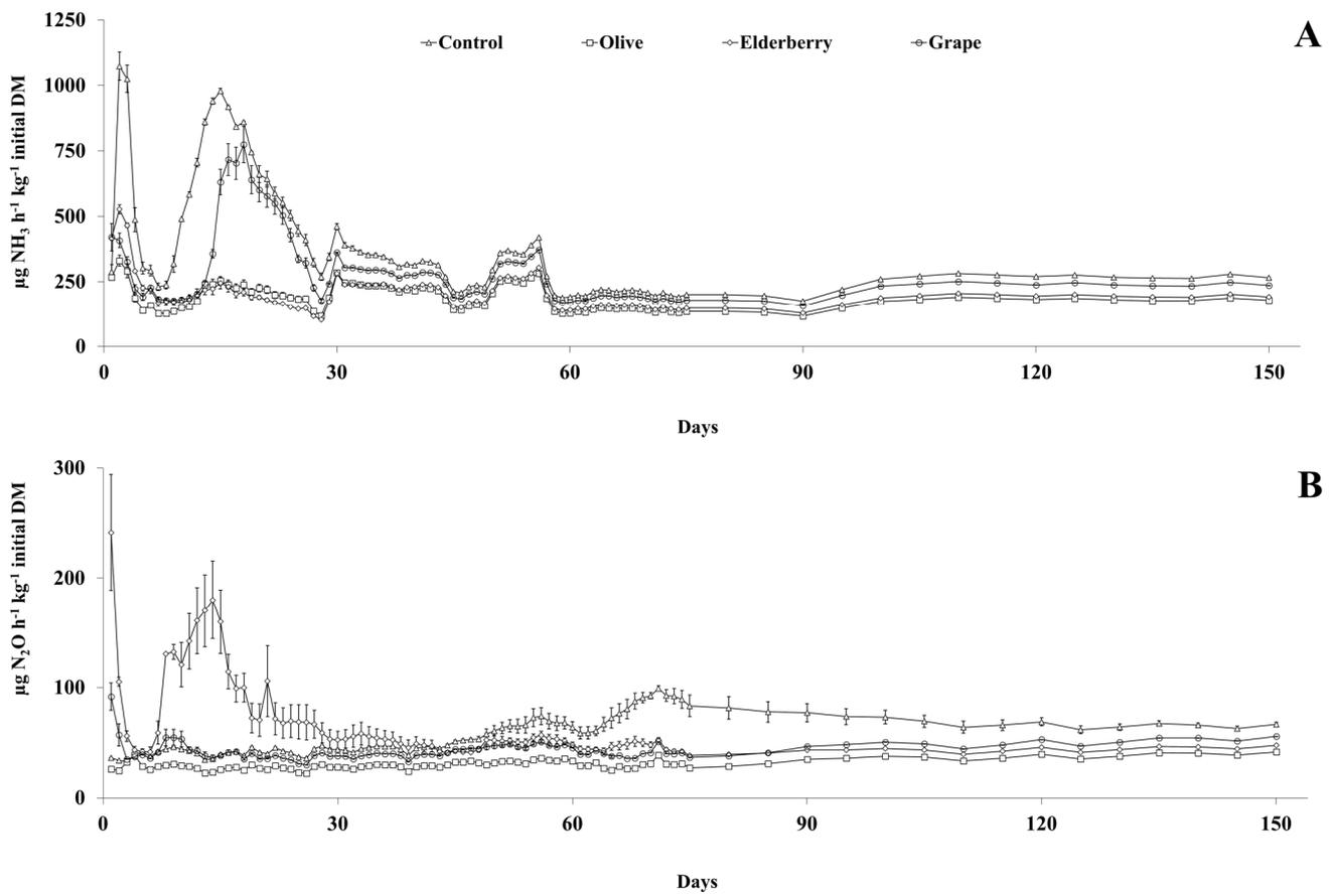
**Figure 5.** Fluxes of  $\text{NH}_3$  (A) and  $\text{N}_2\text{O}$  (B) during the composting experiment treatments. Vertical bars represent standard deviation of 24 h measurements ( $n = 3$ ).
