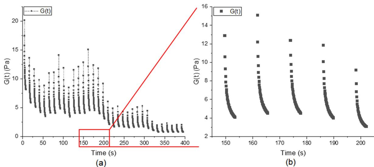
**Figure 4.** (a) Decrease in  $G(t)$  during the relaxation steps for standard wheat flour and water [ $n = 1$ ] as an example of the shear kneading process over the whole 400 s kneading process. (b) Zoom in on the exponential decrease in values for the relaxation steps from 150 s to 200 s kneading time.
