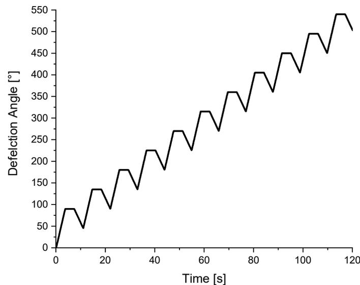
**Figure 1.** Increase in deflection for the kneading procedure with implemented relaxation phases.
