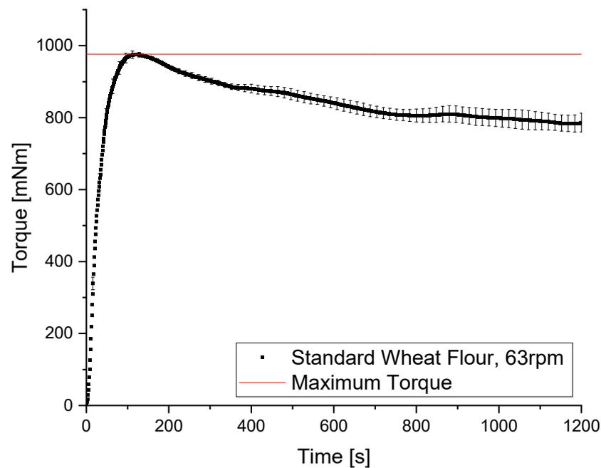
**Figure 2.** Kneading curve for standard wheat flour measured in a torque recording Z-Kneader (DoughLAB). Maximum peak resistance is marked at 976 mNm. Means are shown with standard deviation ( $n = 3$ ).
