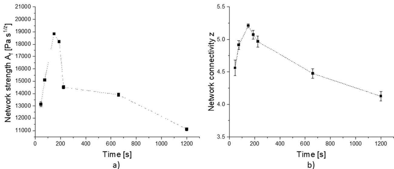
**Figure 3.** (a) Fitting parameter  $A_f$  and (b) parameter  $z$  from power-law fitting the frequency sweep results of dough produced in a Z-Kneader according to Gabriele et al. [19]. Means are shown with standard deviation ( $n = 3$ ).
