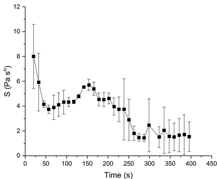
**Figure 5.** Gel strength *S* (fit of the relaxation modulus according to Bhattacharya et al. [24]) calculated from the relaxation steps during the shear kneading process of standard wheat flour and water. Means are shown with standard deviation (*n* = 3).
