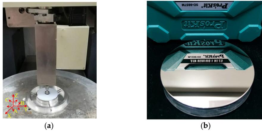
Figure 13.  $\Phi 100$  mm mirror (a) smoothing polishing, and (b) finished mirror.
