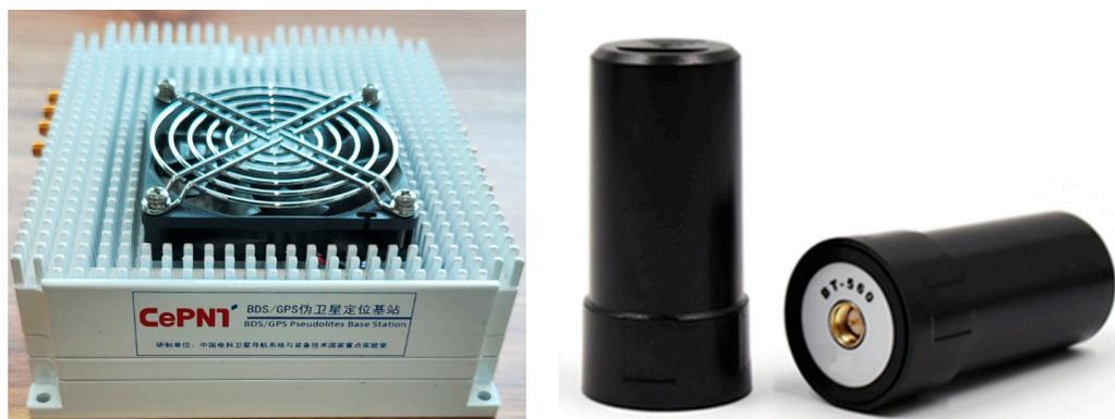
**Figure 1.** Eight-channel indoor array pseudo-satellite base station and transmitting antenna.
