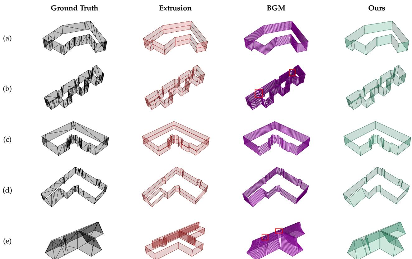
**Figure 18.** Examples of surface-generation results. (a)–(e) show results of five contour pairs from similar to significantly different. The red rectangles show an ambiguous topology generated by bipartite graph matching.
