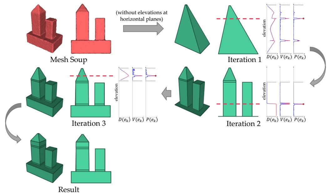
**Figure 4.** An example of the iterative crucial elevation identification with three iterations (without elevations at the horizontal planes here for better explanation). In each iteration, the segment with the largest loss is determined (their boundaries are marked by dashed black lines), and then,  $D(e_k)$ ,  $V(e_k)$ , and  $P(e_k)$  are calculated. The maximum points of  $P(e_k)$  are marked by red circles, and the new elevations are marked by dashed red lines.
