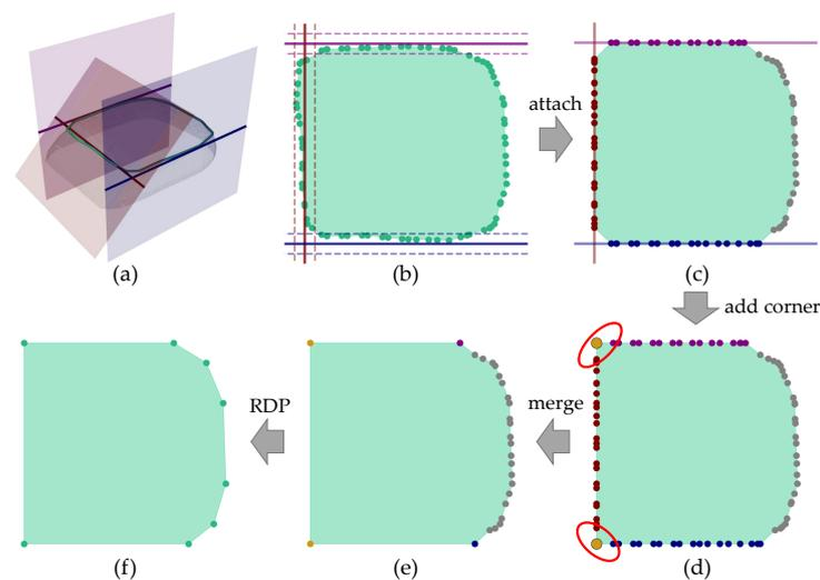
**Figure 6.** An example of contour refinement: (a) Mesh soup, target contour, and three non-horizontal planes with intersected reference lines. (b) Reference lines (solid) and corresponding attach ranges (dashed). (c) Result of vertex attaching. (d) Added corners (orange vertices in red circles). (e) After merging co-linear adjacent edges. (f) Simplified by RDP.
