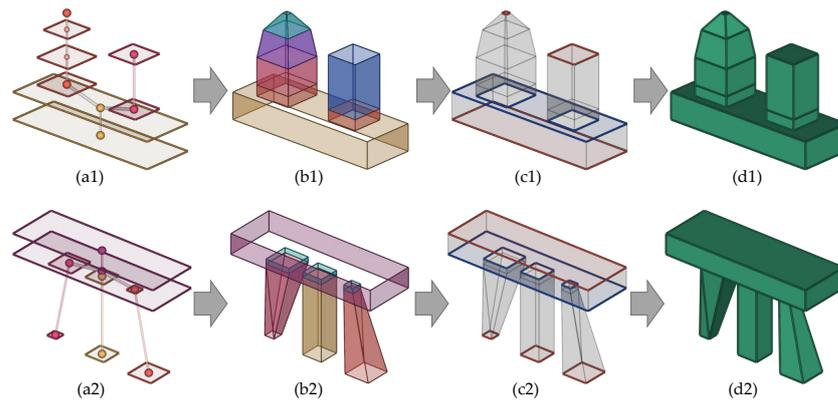
**Figure 8.** Two examples of surface generation: (a1,a2) Refined contour graph (colored by cluster). (b1,b2) Interior faces (colored by node group). (c1,c2) Boundary faces (red for faces from terminal nodes, and blue for faces from 1- $n$  node groups). (d1,d2) generated mesh.
