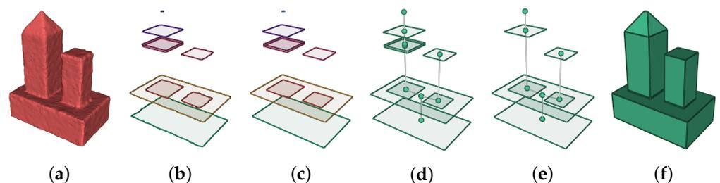
**Figure 2.** Examples of the primary stages in our pipeline: (a) Mesh soup. (b) Vital contour layers with raw contours. (c) Contour layers after the refinement of contours. (d) Contour graph. (e) Contour graph after removing two redundant contours in the post-processing. (f) Final reconstructed mesh.
