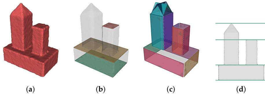
**Figure 3.** An example of the extracted planes and initial crucial elevations: (a) Mesh soup. (b) Horizontal planes of buildings. (c) Non-horizontal planes of buildings. (d) Initial crucial elevations.
