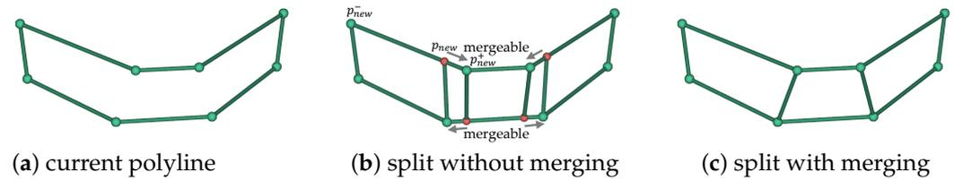
**Figure 10.** An example of polyline splitting with and without vertex merging.
