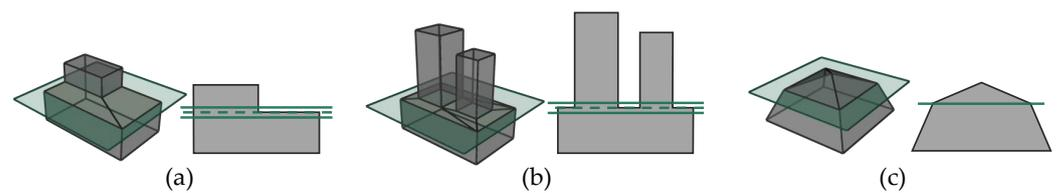
**Figure 5.** Contour layer extraction in different circumstances. The green planes and dashed green lines refer to the current elevations, and the solid green lines indicate the elevations of the added contour layers. (a,b) have dramatic topological variations, and two contour layers are added. (c) has a smooth variation, and thus, only one contour layer is added.
