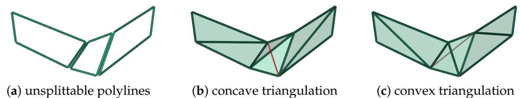
**Figure 11.** Concave and convex triangulation of non-planar quadrilateral polylines. The red edge indicates the other triangulation result of the middle polyline for comparison.
