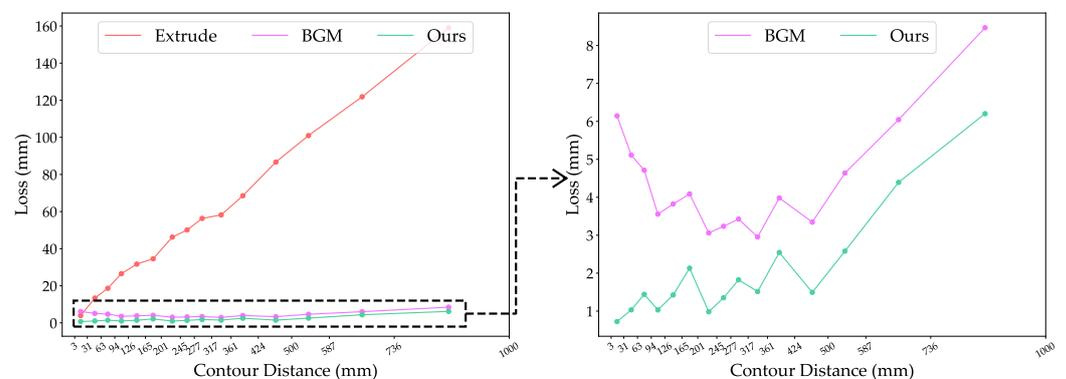
**Figure 19.** The average losses of surface-generation results at different ranges of contour distances for data in the “different-pair” part. The left subfigure shows the results of extrusion, BGM, and our method, while the right subfigure only shows the results of BGM and our method for better clarity.
