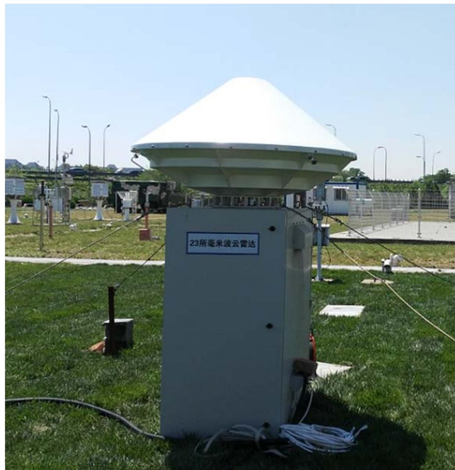
**Figure 1.** Photo of HMB-KPS millimeter-wave radar.
