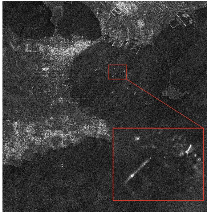
**Figure 9.** Test case of the CFAR+SLA algorithm over the port of Taranto. Highlighted detail: a probable radio signal transmitted from a ship and captured by X-band spaceborne SAR. Product ID: CSKS1\_SCS\_BHI\_05\_HH\_RD\_SF\_20200323164522\_2020032316\_4529, processed by University of Naples Federico II under the COAST license of the Italian Space Agency (ASI). Original COSMO-SkyMed Product ©ASI (2020).
