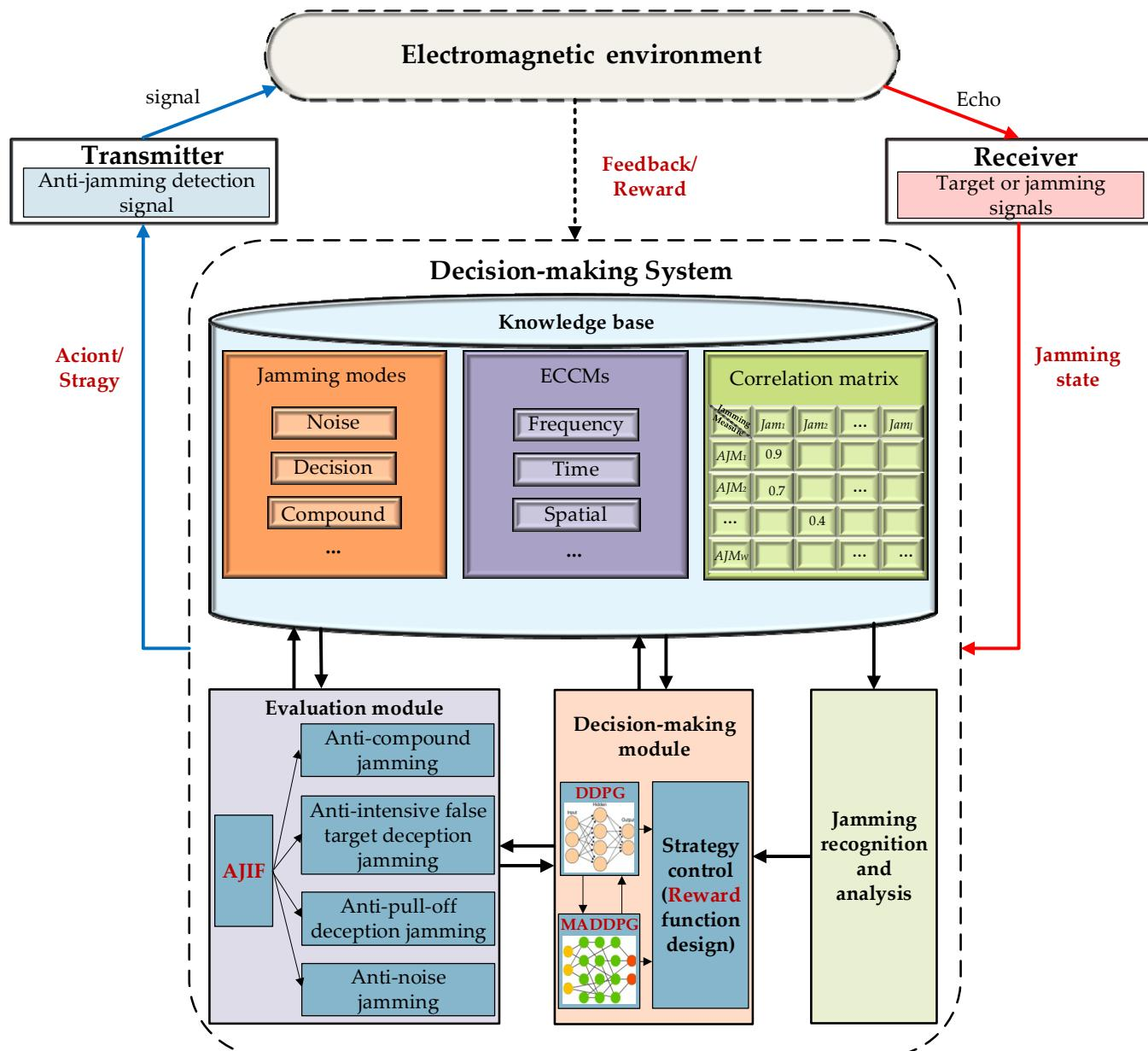
Figure 2. Intelligent radar anti-jamming decision-making model.
