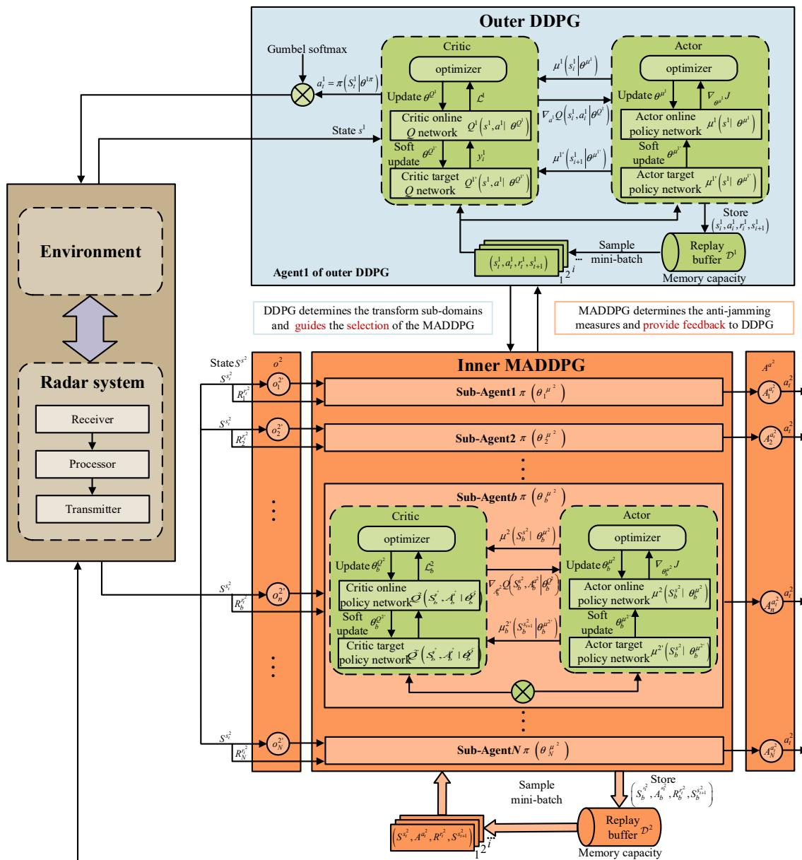
**Figure 3.** The dual RL model of DDPG-MADDPG.
