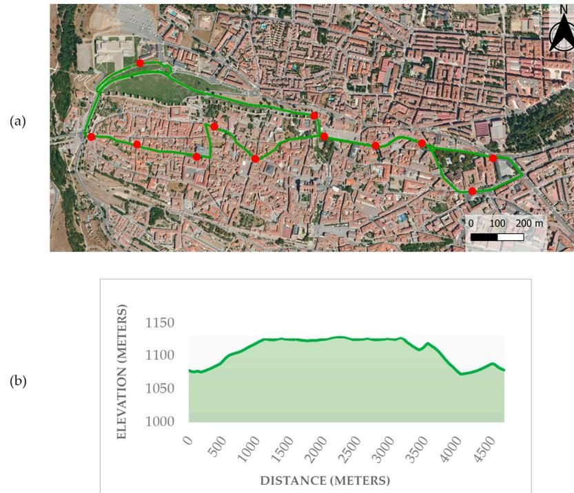
**Figure 12.** Possible route, option 1: (a) bus trajectory with strategic points; (b) topographical profiles obtained from the DEM (point cloud with 1 point/m<sup>2</sup>).
