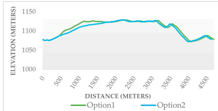
Figure 14. Topographical profiles obtained from the DEM (point cloud with 1 point/m<sup>2</sup>): option 1 vs. option 2.
