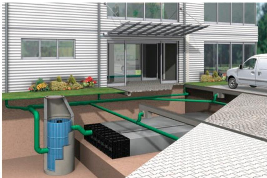
**Figure 7.** Typical filter shaft with underground storage and infiltration facility [34].
