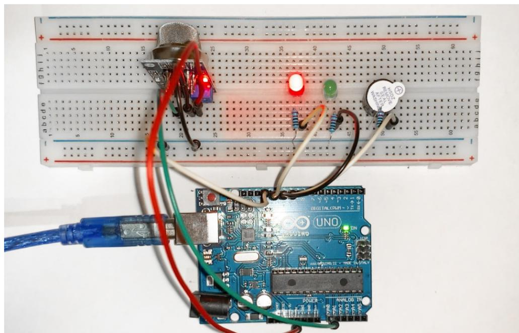
**Figure 11.** Scheme of the model when the threshold value of methane concentration is exceeded by the MQ-4 sensor; the red LED lights up. Source: Compiled by the author.
