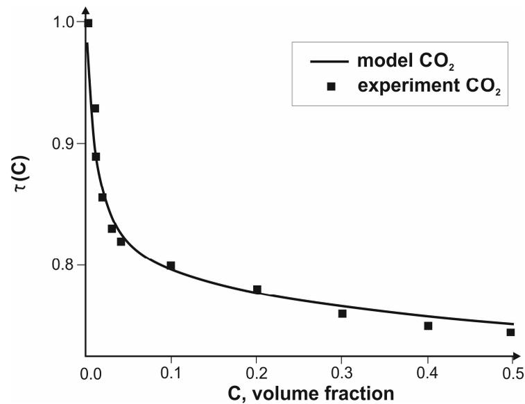
Figure 4. Transfer functions for the CO<sub>2</sub> sensors.
