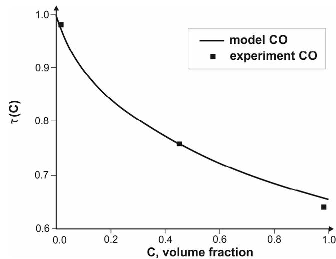
Figure 5. Transfer functions for the CO sensors.
