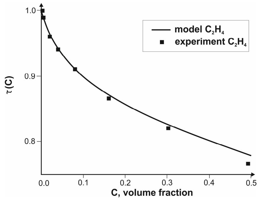
Figure 6. Transfer functions for the  $C_2H_4$  sensors.
