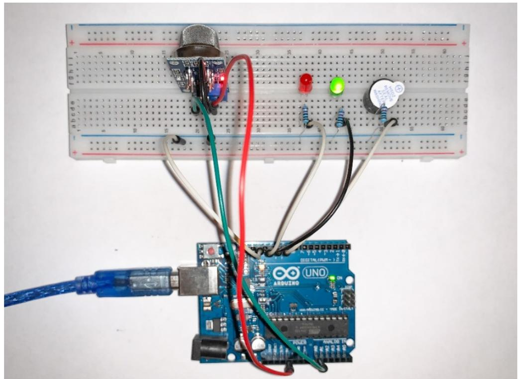
Figure 10. Diagram of the model at a normal value of methane concentration; the green LED lights up. Source: Compiled by the author.
