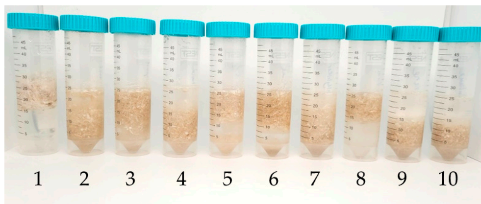
Figure 6. Partitioning properties of duck feathers between air and the different solvents, solvent (1) water, (2) ethanol, (3) isopropanol, (4) acetone, (5) acetonitrile, (6) toluene, (7) diethyl ether, (8) chloroform, (9) hexane, and (10) pentane.
