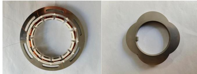
**Figure 18.** Prototype of the produced resolver.
