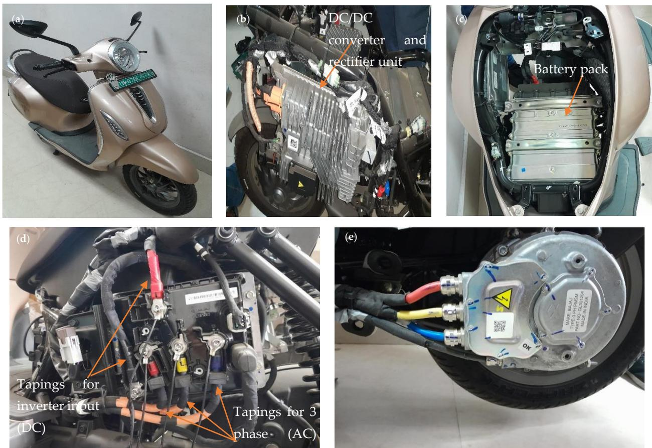
**Figure 1.** (a) Vehicle under test, (b) DC/DC converter and rectifier unit, (c) sealed battery pack, (d) inverter and motor control unit, and (e) three-phase PMSM.
