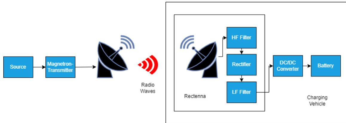
**Figure 11.** A radio wave charging system.
