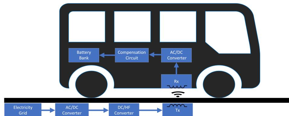
**Figure 1.** General structure of a static wireless charging system for EVs. The coils may be replaced by capacitive pads in capacitive coupling.
