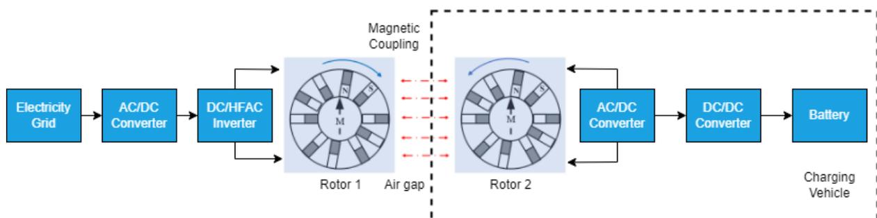
**Figure 8.** Architecture of an MGWPT system.
