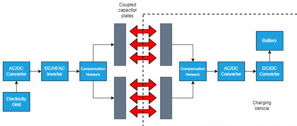
Figure 5. Structure of a CPT system.
