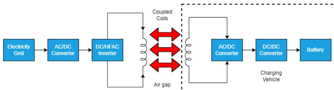
Figure 6. Structure of an IPT system. Compensation networks can be added before the primary and after secondary windings.
