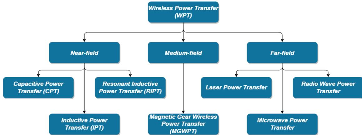
**Figure 3.** All wireless power transfer methods mentioned in the literature relevant to wireless EV charging.
