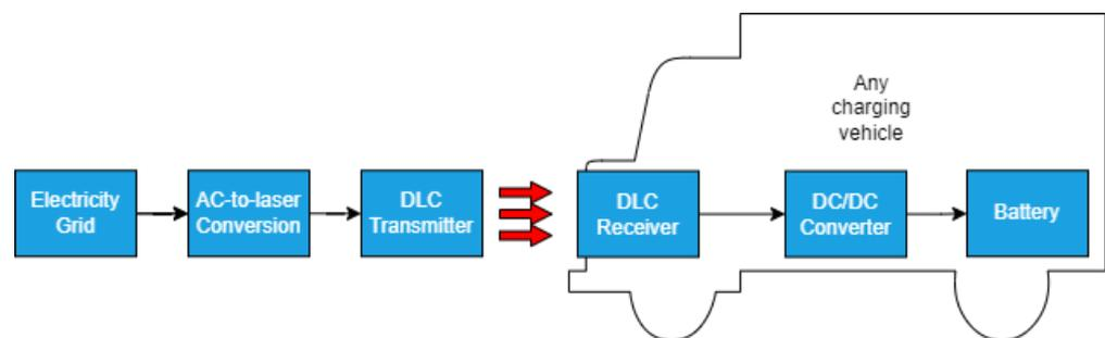
**Figure 9.** A laser charging system.
