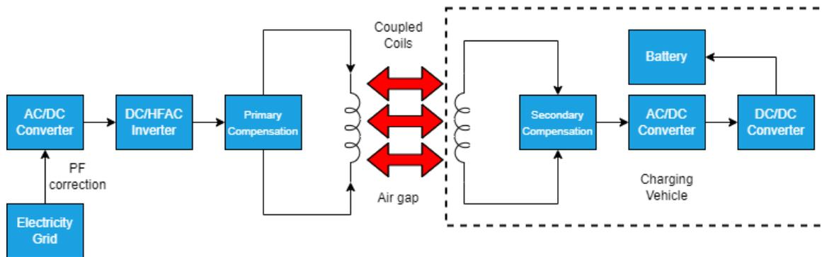
**Figure 7.** Structure of a RIPT system, an enhanced version of an IPT system.
