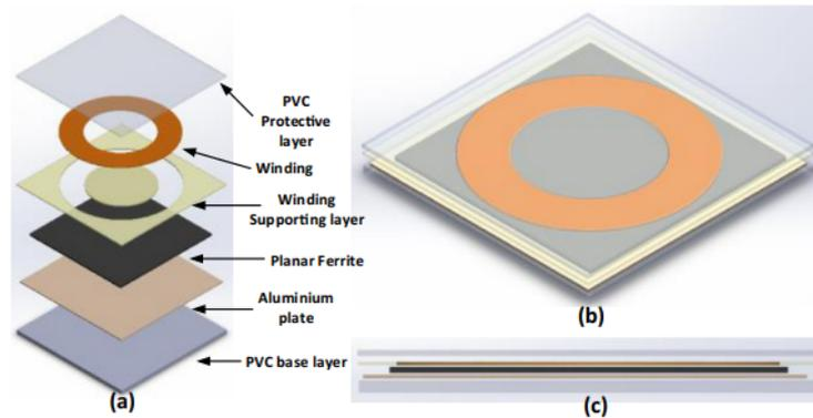
**Figure 12.** Typical structure of an IPT charging pad [4]: (a) exploded view, (b) top view, and (c) side view.
