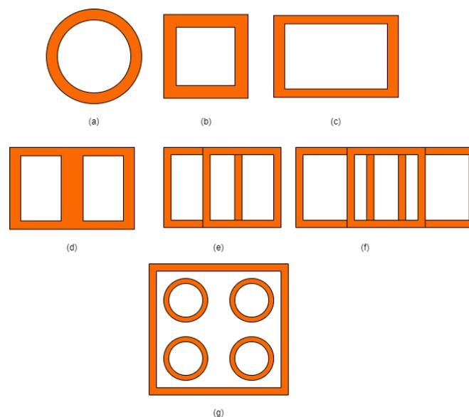
**Figure 13.** Various coil shapes that are typically used: (a) circular, (b) square, (c) rectangular, (d) DD, (e) BP, (f) DDQ, and (g) QDQ.
