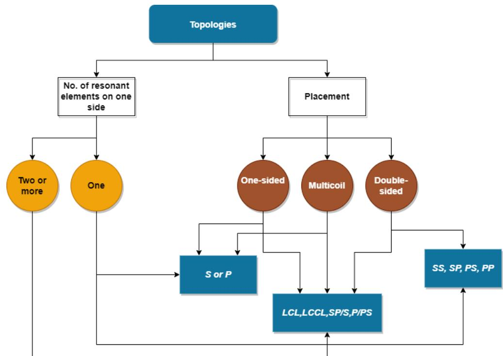
**Figure 15.** Classification of compensation topologies based on the number of resonant elements in either the transmitter or receiver and the location in the system.
