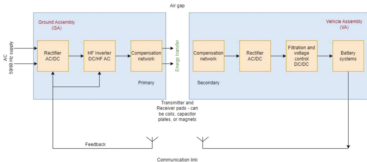
**Figure 4.** The common architecture of a WPT system.
