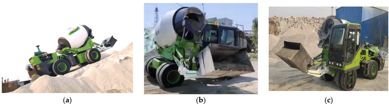
**Figure 20.** Experimental verification of working condition b. (a) Mixer truck uphill 15 degrees and bucket flat. (b) Mixer truck with upper load rotated 90 degrees and bucket flat. (c) Mixer truck at rest with the bucket flat.
