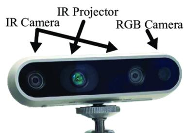
**Figure 4.** Illustration of an Intel RealSense D435 camera with an infrared projector, a color (RGB) camera, and two cameras to collect stereo depth (D) images.
