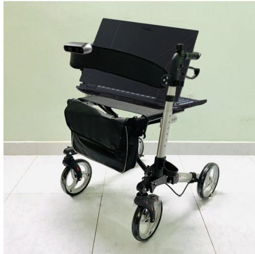
**Figure 5.** Illustration of a vehicle equipped with a camera and computer when collecting data.
