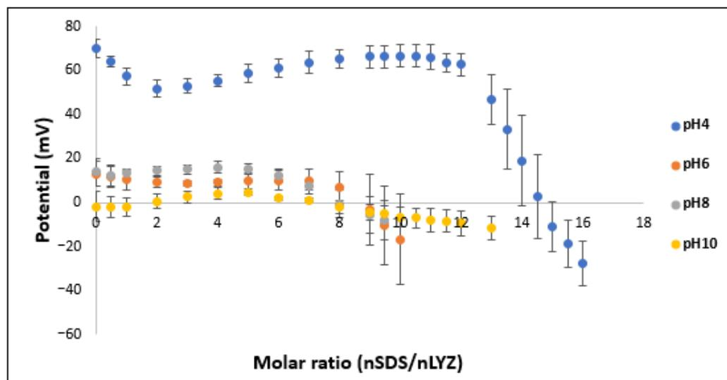
**Figure 3.** Titration curve representing the change in streaming potential (mV) upon the addition of small increments of a 7  $\mu$ M SDS solution to a 2 mg/mL LYZ solution at pH 4, 6, 8 and 10. The intersection of the curves with a zero potential line represents the average SDS/LYZ molar ratios of three measurements at the neutralization point.
