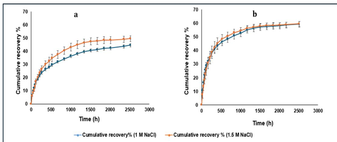
**Figure 6.** Cumulative recovered amount of LYZ from the complexes prepared at pH 6 (a) and 8 (b) upon addition and incubation in 1 M and 1.5 M NaCl solutions (average of five measurements).
