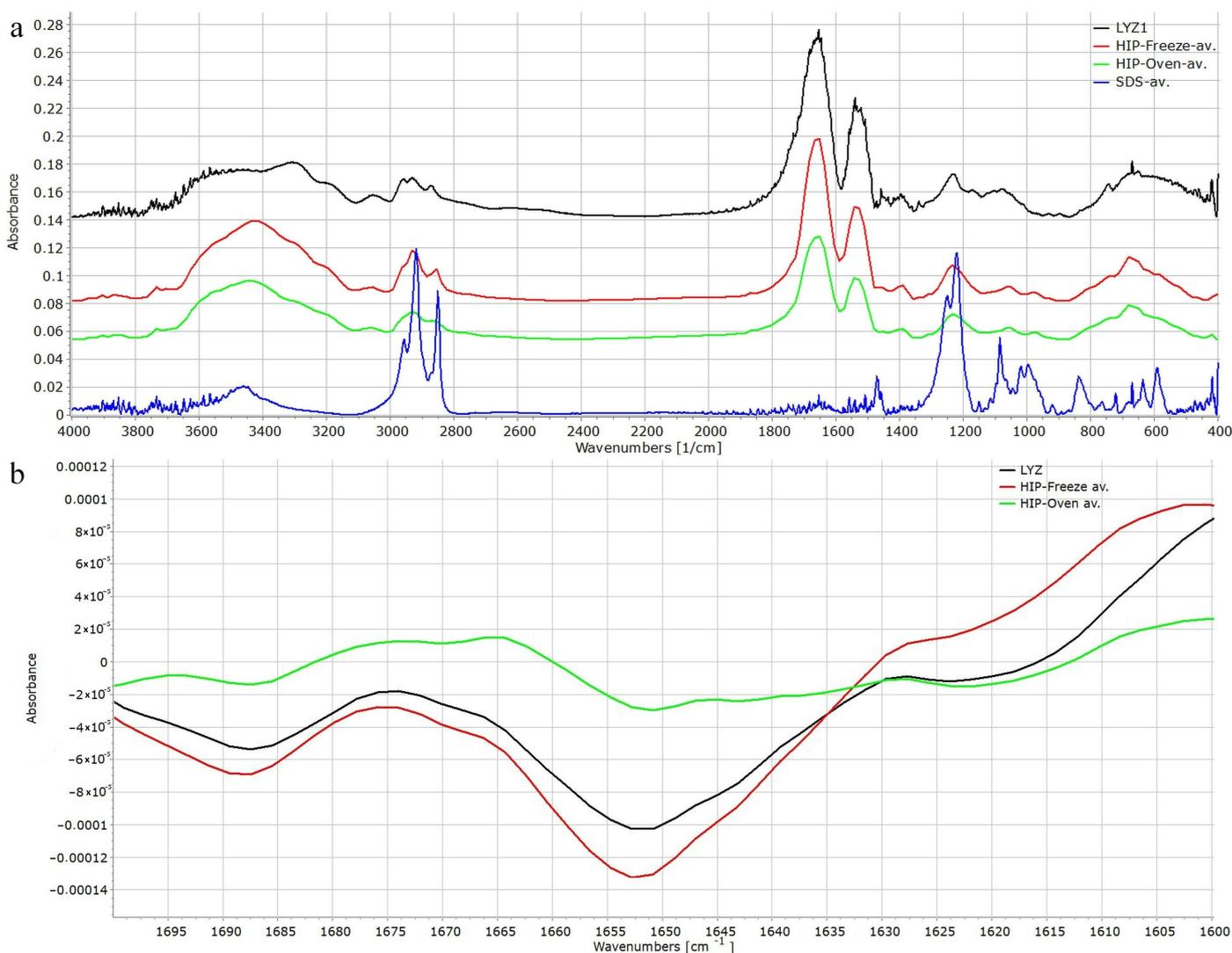
**Figure 10.** FTIR spectra of SDS, LYZ, freeze-dried HIP and oven-dried HIP complex of LYZ and SDS. (a) The second derivative of the amide I peak of LYZ, freeze-dried HIP and oven-dried HIP complex of LYZ and SDS (b).
