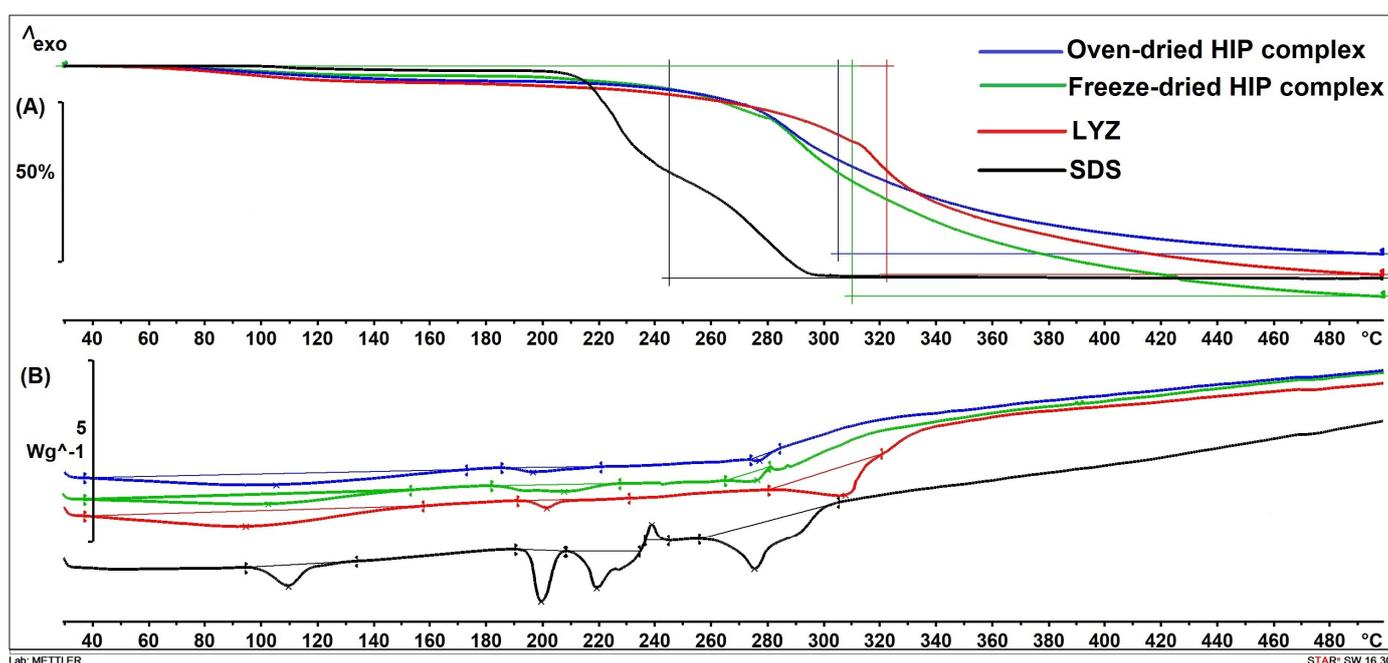
**Figure 11.** Thermograms of SDS, LYZ, freeze-dried HIP and oven-dried HIP complex of LYZ and SDS: (A) TGA thermogram, (B) DSC thermogram.
