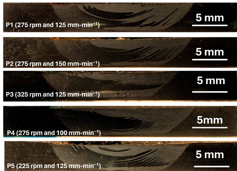
Figure 2. Macrographs of transverse cross-sections of friction stir-welded dissimilar alloys: Ti-54M (RET) and Ti-6242-SG (ADV).
