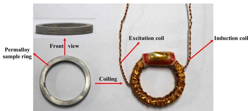
**Figure 2.** Schematic diagram of permalloy sample ring.
