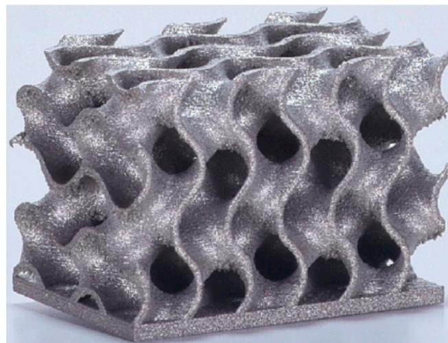
**Figure 6.** View of the gyroid structure made using the AM method for the study of heat transfer under forced convection conditions [83].
