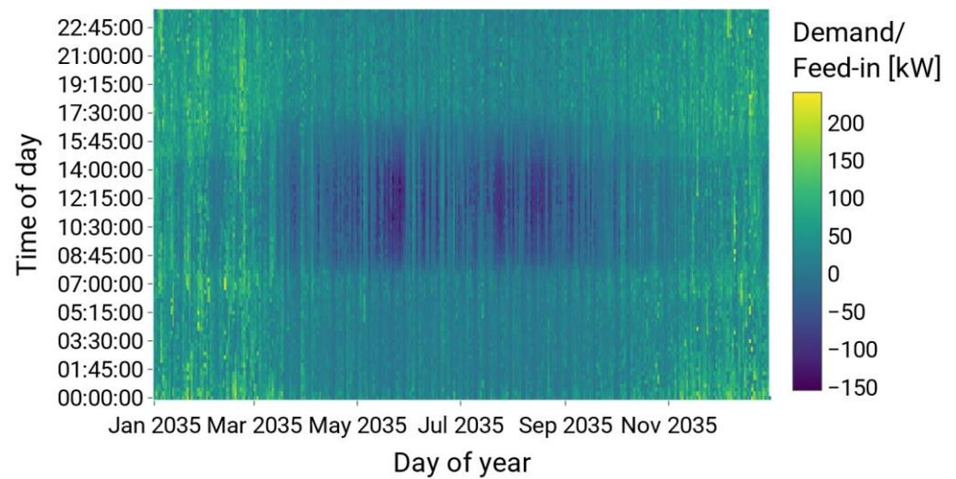
**Figure A2.** Heatmap of the electric demand (positive values) and feed-in (negative values) for the flat participant fee scenario, the scenario year 2035 and the rural grid.
