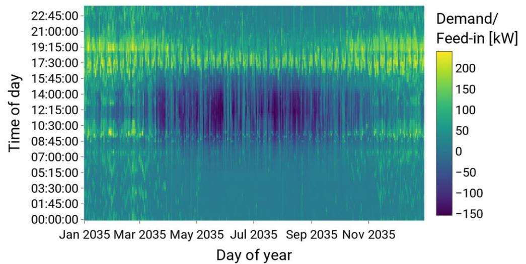
**Figure 6.** Heatmap of the electric demand (positive values) and feed-in (negative values) for the business-as-usual scenario, the scenario year 2035 and the rural grid.
