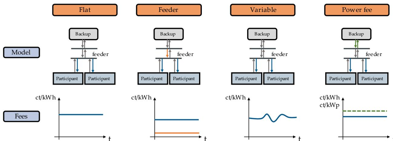
**Figure 3.** Overview of analyzed grid tariff models for LEMs. Lines and arrows: blue—participant energy fees ct/kWh; orange—feeder energy fees ct/kWh; green—power fees ct/kWp.
