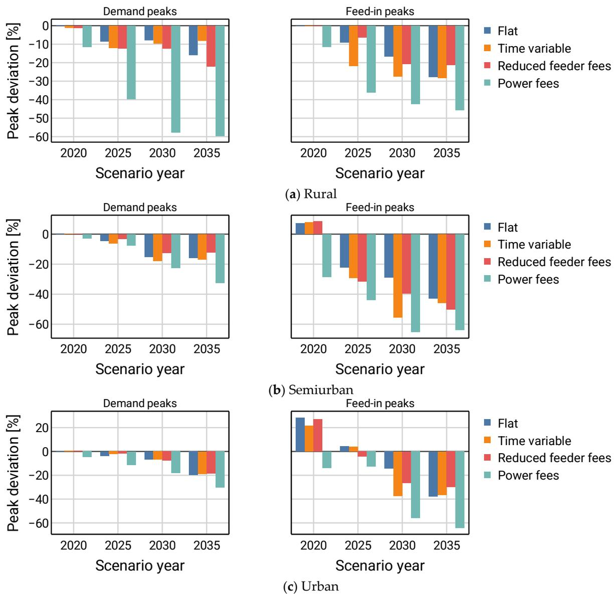
**Figure 9.** Relative deviation of demand and feed-in peaks for a variation of grid types (a–c) and scenario years and grid tariff designs. Deviation calculated using the 5% highest daily peaks of the business-as-usual scenario.
