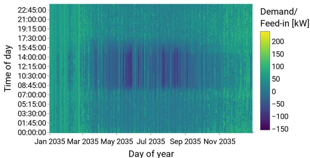
**Figure A4.** Heatmap of the electric demand (positive values) and feed-in (negative values) for the power fee scenario, the scenario year 2035 and the rural grid.
