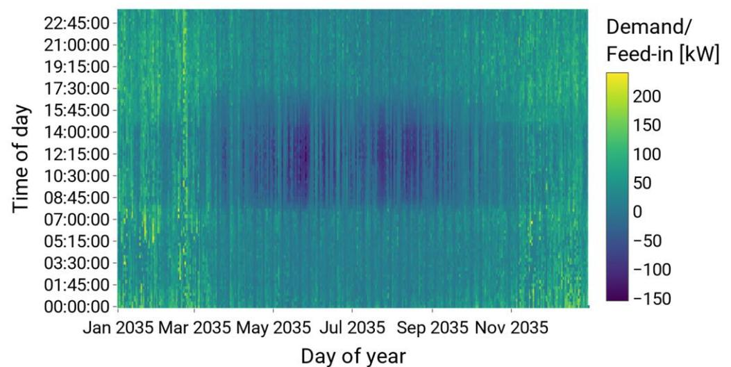
**Figure 7.** Heatmap of the electric demand (positive values) and feed-in (negative values) for the scenario with time variable fees, the scenario year 2035 and the rural grid.
