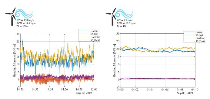
**Figure 10.** Experimental and numerical bending moments time series for FA and SS directions in the bottom-instrumented section of the tower considering two different operating conditions.
