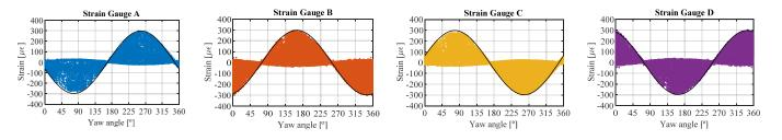
Figure 8. Ten-minute average strain signal of strain gauges A to D (see sensor positions in Figure 4c).
