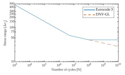
Figure 2. S-N curves defined in GL-2010 and Eurocode 3 (category detail 80 MPa).
