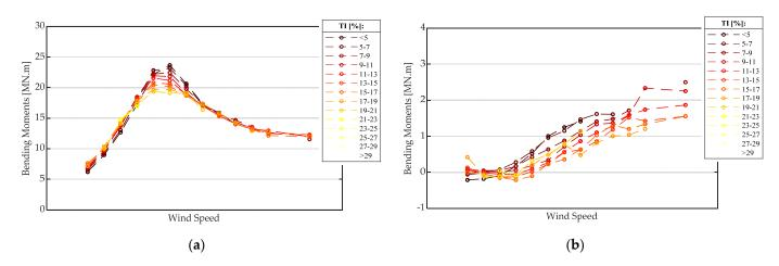
**Figure 11.** Variation of 10 min average bending moments at the tower base as a function of the wind speed and turbulence intensity, considering normal power production: (**a**) fore–aft direction, and (**b**) side-to-side direction (x scale omitted because of confidentiality agreements).
