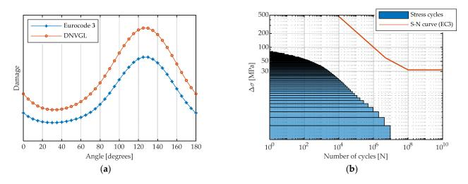
**Figure 14.** Influence of the S-N curve parameters: (**a**) damage distribution over the section (y scale omitted due to confidentiality agreements); and (**b**) histogram of the stress cycles and S-N curve provided by Eurocode 3.
