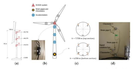
**Figure 4.** Tower monitoring systems: (a) sections instrumented with force balance accelerometers; (b) force balance sensors S1 and S2; (c) strain and rotation monitoring system; and (d) position of the strain gages ( $\Diamond$ ) and temperature sensors ( $\bigcup^{+}$ ) at the tower.
