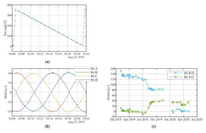
**Figure 7.** Strain-gauge calibration check: (**a**) yaw angle nacelle; (**b**) strain signals; and (**c**) mean value of the full rotation signals observed from February 2019 to April 2020 (see sensor positions in Figure 4c).
