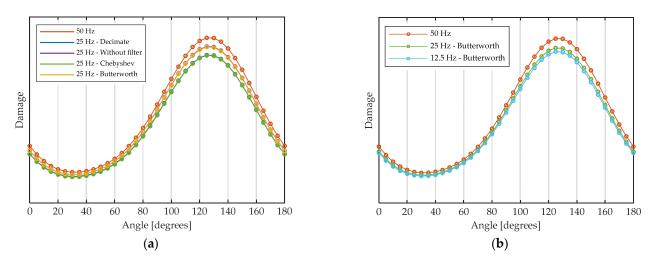
**Figure 16.** Influence of signal sampling frequency: (a) damage distribution over the section considering tree methods ( $f_s = 25$  Hz); and (b) damage distribution over the section for all sampling frequency (Butterworth filter). Y scale omitted because of confidentiality agreements.
