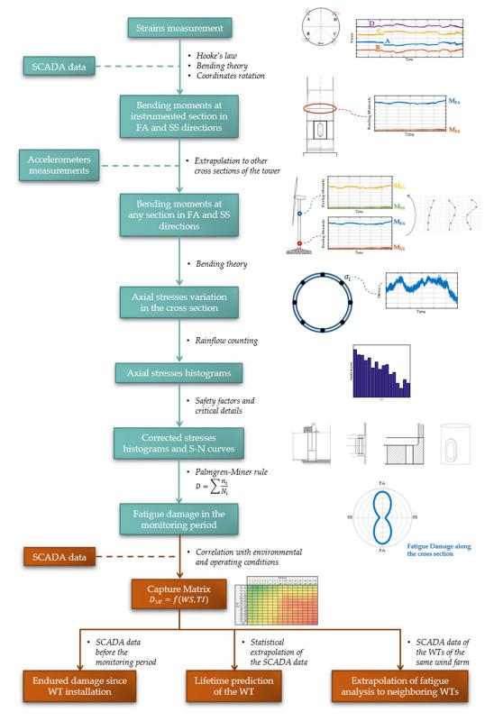
Figure 1. Fatigue assessment procedure based on strain measurements.
