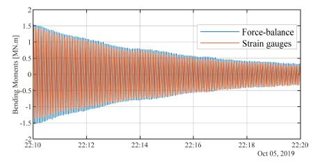
**Figure 9.** Bending moment variations at the base of the tower estimated from acceleration and strain time series during a rotor stop event.
