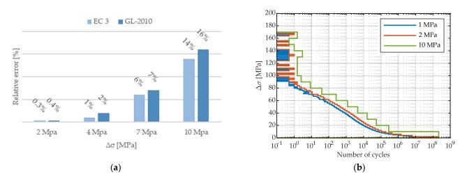
**Figure 13.** Influence of the rainflow histogram resolution: (**a**) relative difference of the calculated damage (the 1 MPa bin amplitude is the reference); and (**b**) stress cycles histogram.
