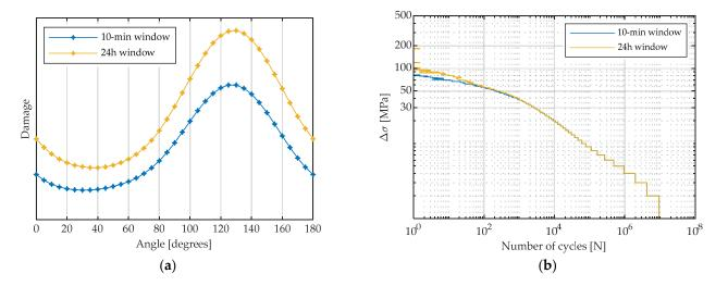
**Figure 12.** Influence of the window length: (**a**) damage distribution over half of the section (y scale omitted due to confidentiality agreements); and (**b**) histogram of the stress cycles.
