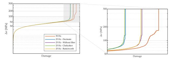
**Figure 15.** Influence of signal sampling frequency. Stress cycles as a function of the accumulated damage for a sampling frequency of 25 Hz, with zoom (x scale omitted because of confidentiality agreements).
