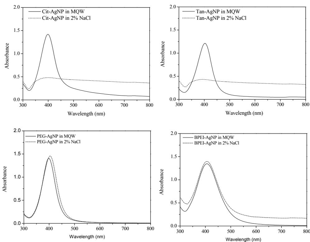
**Figure 1.** UV-Vis absorption spectrum peaks of surface-coated AgNPs in both MilliQ water only (straight line) and 2% NaCl solution (dashed line).
