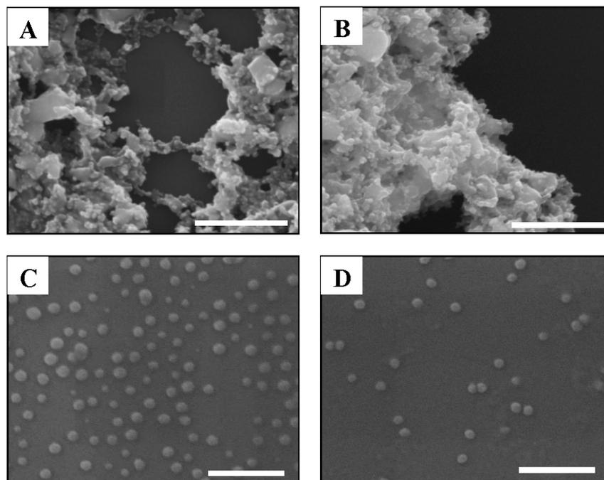
**Figure 2.** SEM images of surface-coated AgNPs in 2% NaCl solution. (A and B) Aggregation of both citrate (Cit)-AgNPs and tannic acid (Tan)-AgNPs in 2% NaCl solution and (C and D) non-aggregation of both polyethylene glycol (PEG)-AgNPs and branched polyethylenimine (BPEI)-AgNPs in 2% NaCl solution. (Scale bar = 200 nm)
