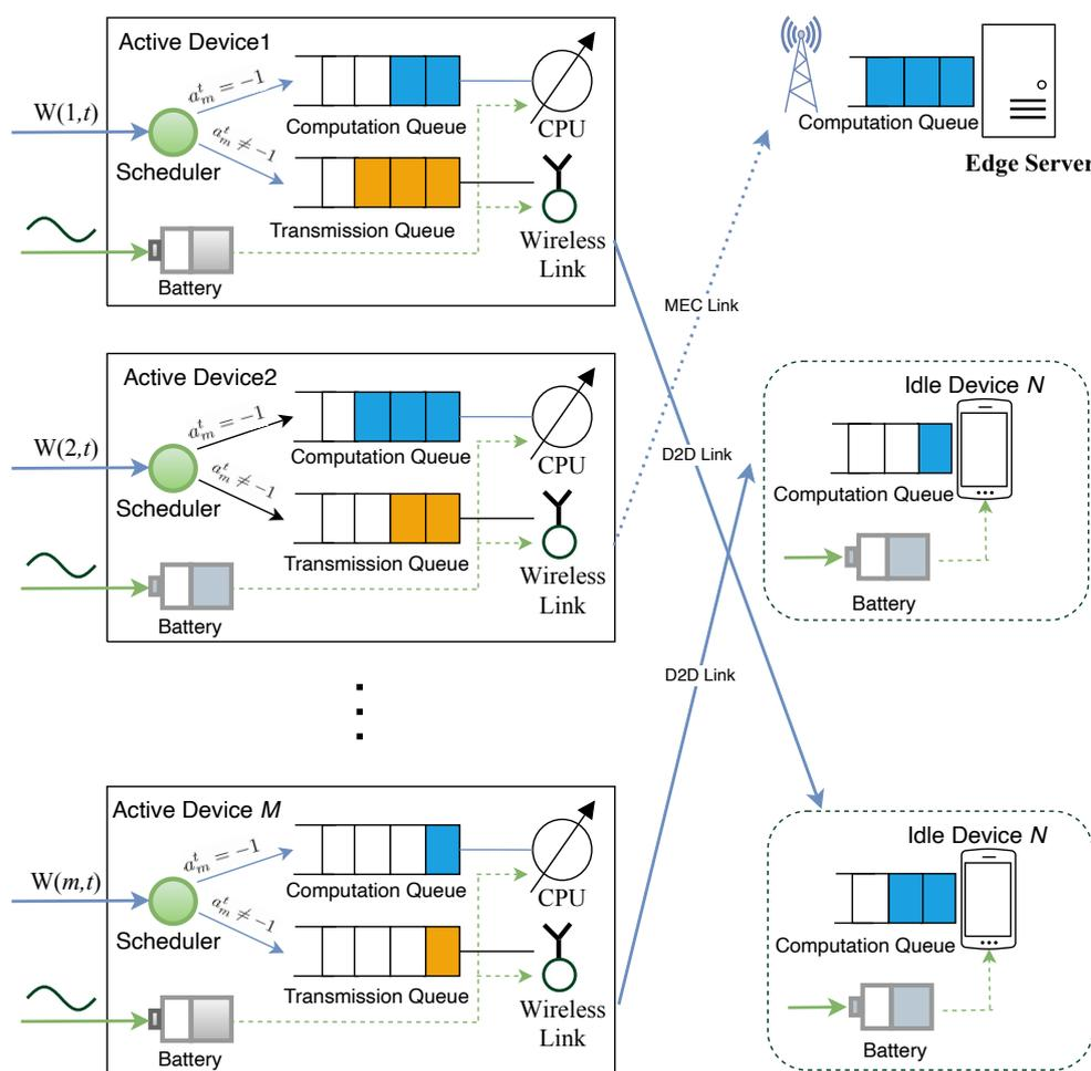
Figure 1. Architecture of D2D-MEC network.
