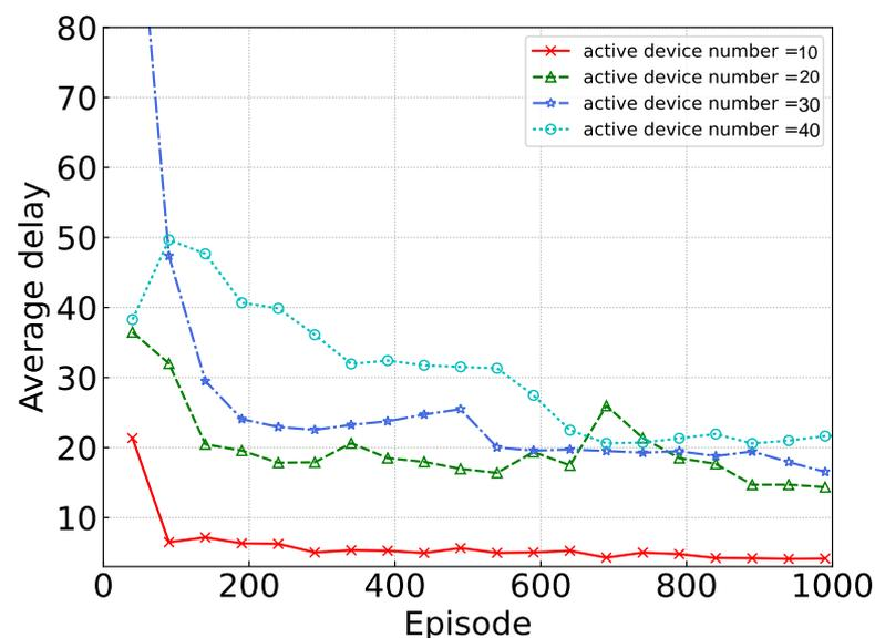
**Figure 5.** Convergence under different numbers of active devices.
