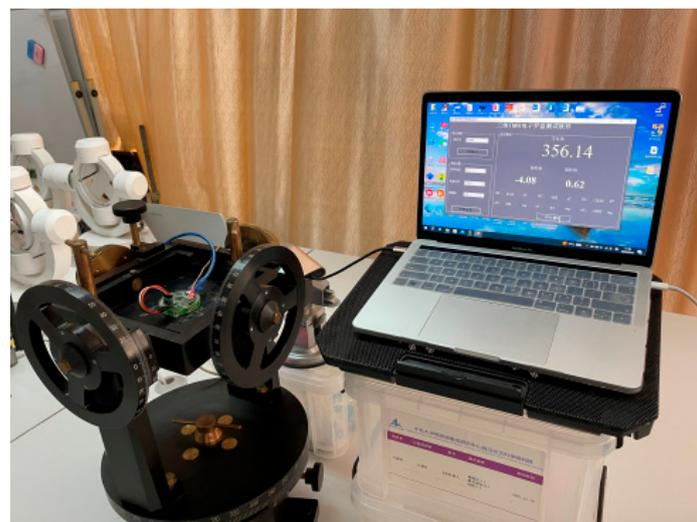
**Figure 11.** Schematic diagram of digital compass precision test platform.
