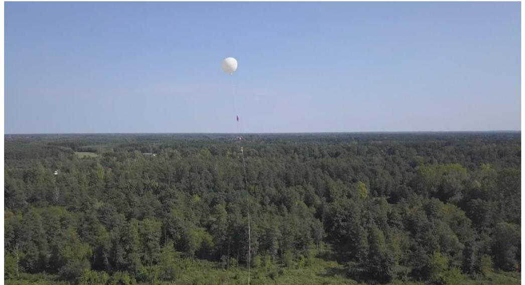
**Figure 5.** An example of the launch of a light stratospheric balloon mission (12 September 2018) with the deployment of a 40 m-long vertical antenna; seen from the top: the balloon, the parachute, the main gondola, the antenna fixing insulator and the antenna (aluminum tape-form) during deployment.
