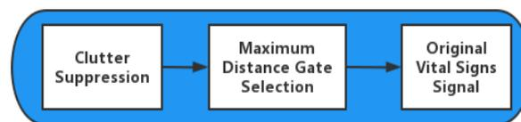
Figure 2. Radar echo preprocessing process.
