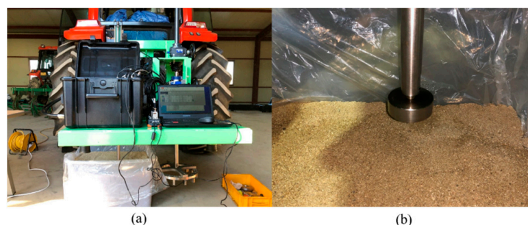
Figure 8. Pressure–sinkage test in the sample soil: (a) setup and (b) test in progress.
