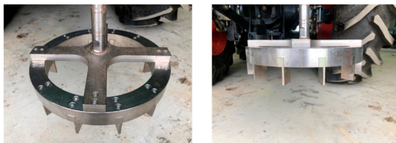
Figure 6. Shear ring with grousers placed at intervals of 30^\circ .
