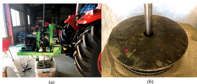
Figure 9. Shear test with the sample soil: (a) setup and (b) test in progress.
