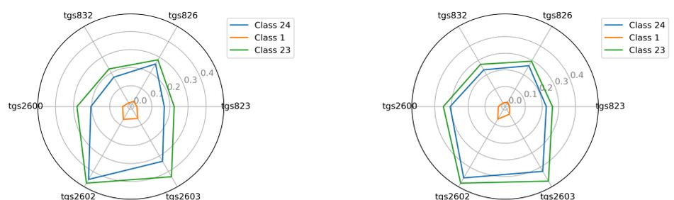
**Figure 7.** The visualization of the average reading intensity of TGS sensors for decision classes 1, 23, and 24 using M1; wooden chamber on the left and polystyrene chamber on the right.
