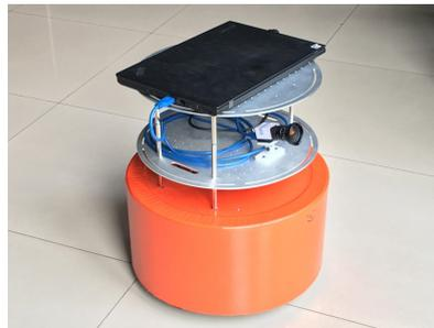
Figure 5. Redbot with a daheng monocular camera.
