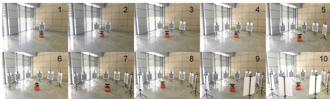
**Figure 12.** Experimental setup to test the effect of the number of the targets on calibration results.
