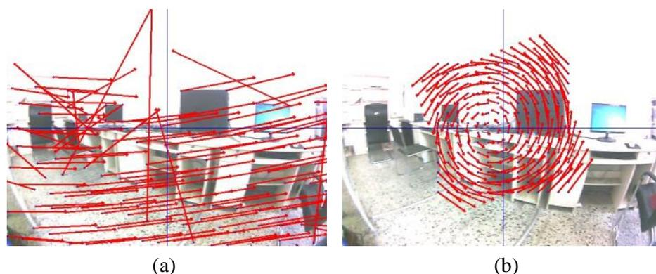
**Figure 6.** The motion flow at  $\omega_z^{cam} = -2.82$  rad/s (a) a KLT tracker and (b) an IMU-aided motion estimator.
